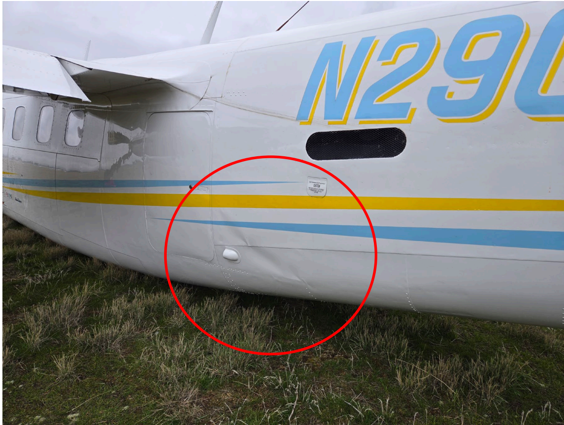
Photograph 2 - View of fuselage buckling (Courtesy of Airport Operations)
