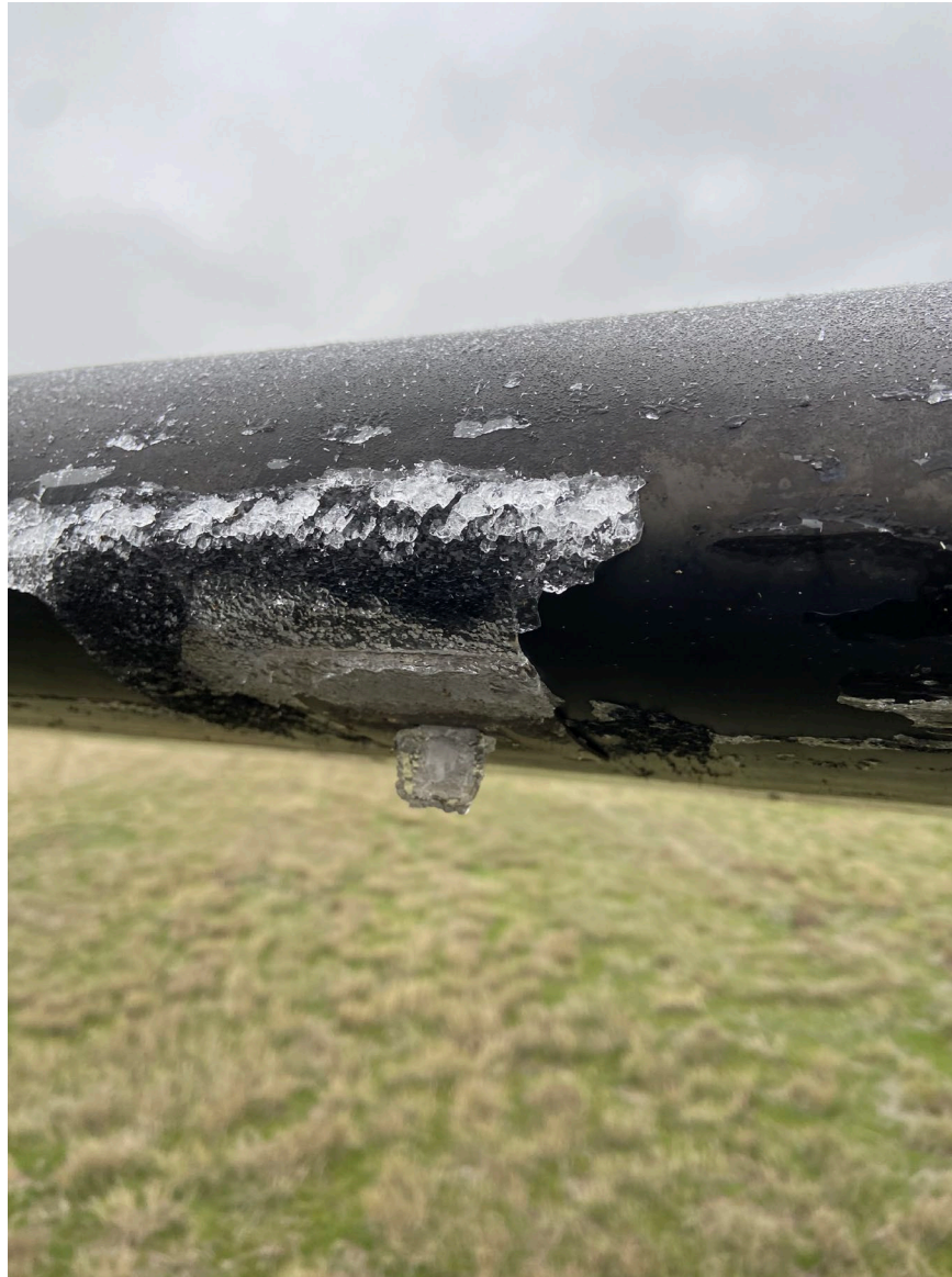
Photograph 4 - View of ice on stall warning (Courtesy of FAA)
