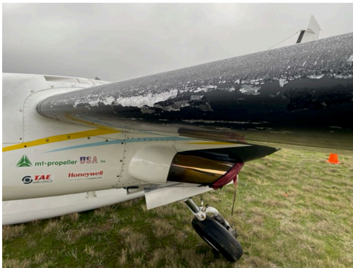
Photograph 5 - View of ice on leading edge of wing (Courtesy of FAA)
