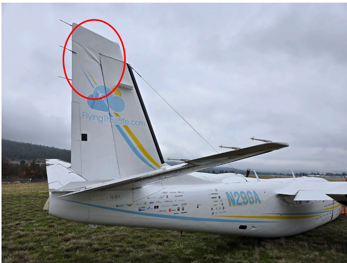
Photograph 3 - View of rudder damage (Courtesy of Airport Operations)
