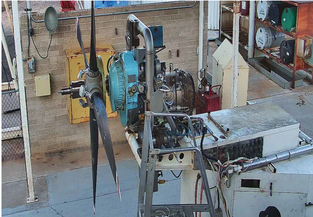
Figure 8: View of right engine on test stand.
