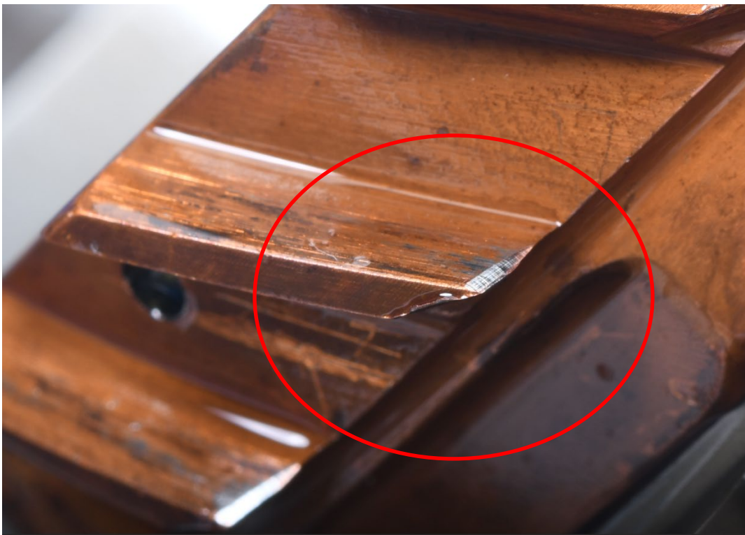
Figure 5: View of damage to helical spline teeth on the helical cam gear shaft (left engine).
