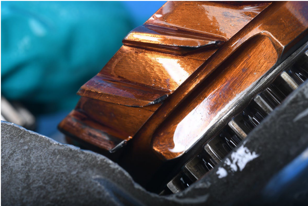
Figure 10: View of damage to helical spline teeth on the helical cam gear shaft (right engine).
