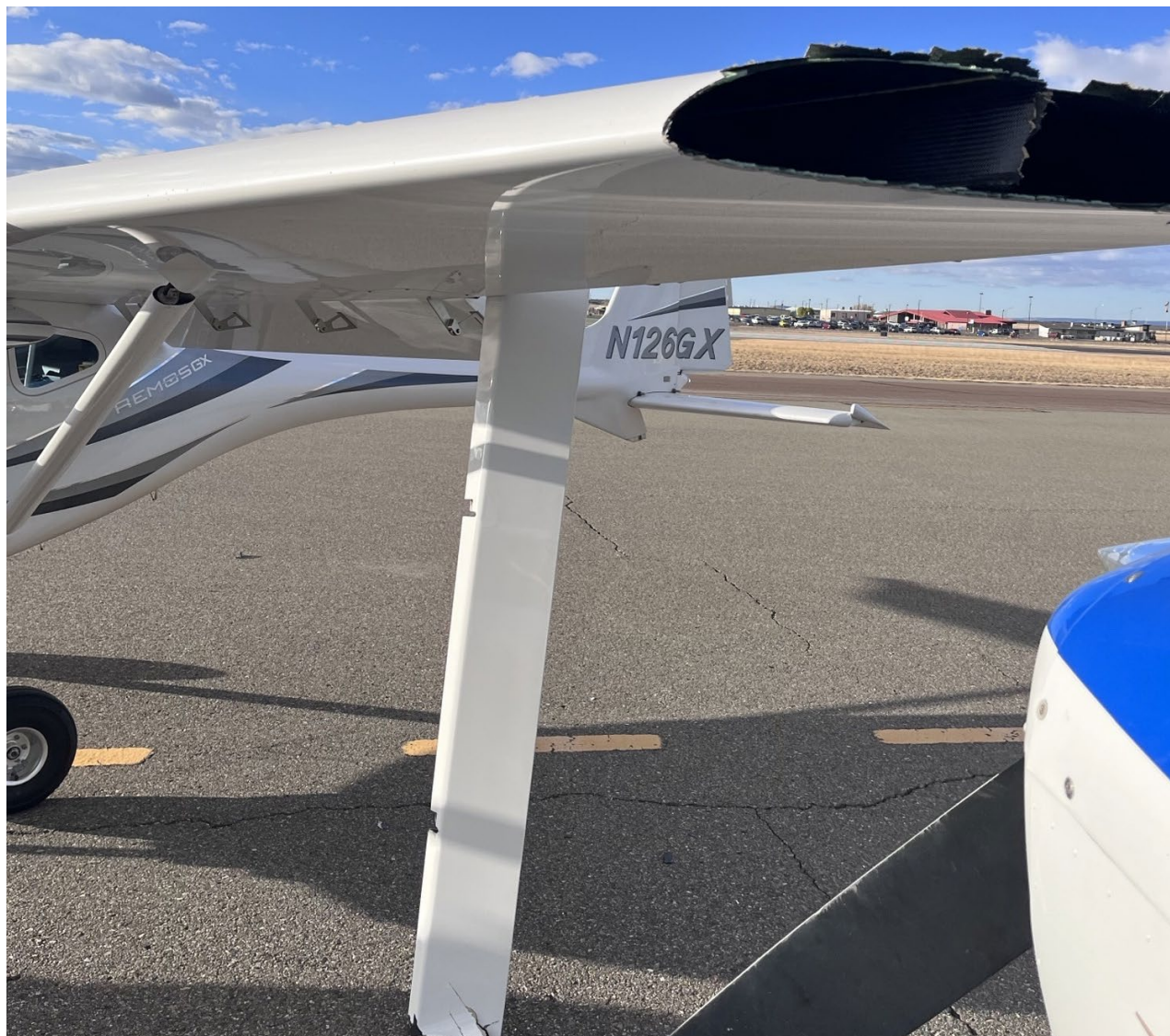
Photograph 1 - Substantial Damage of Remos Wing (Courtesy of ERAU)
