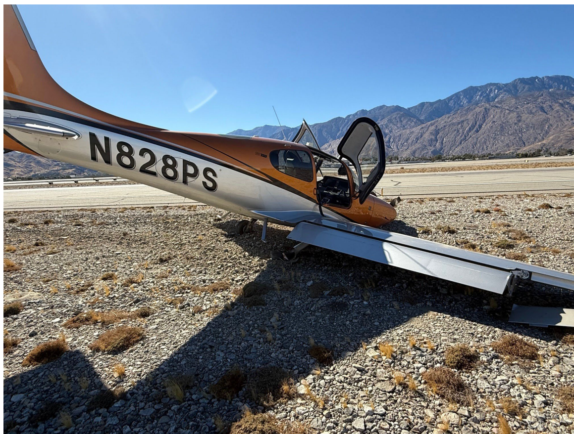
Photograph 2 - Substantial damage to right aileron (Courtesy of pilot)
