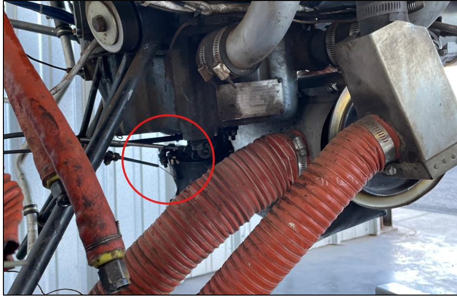
Figure 4-Separated mixture cable near the carburetor.
