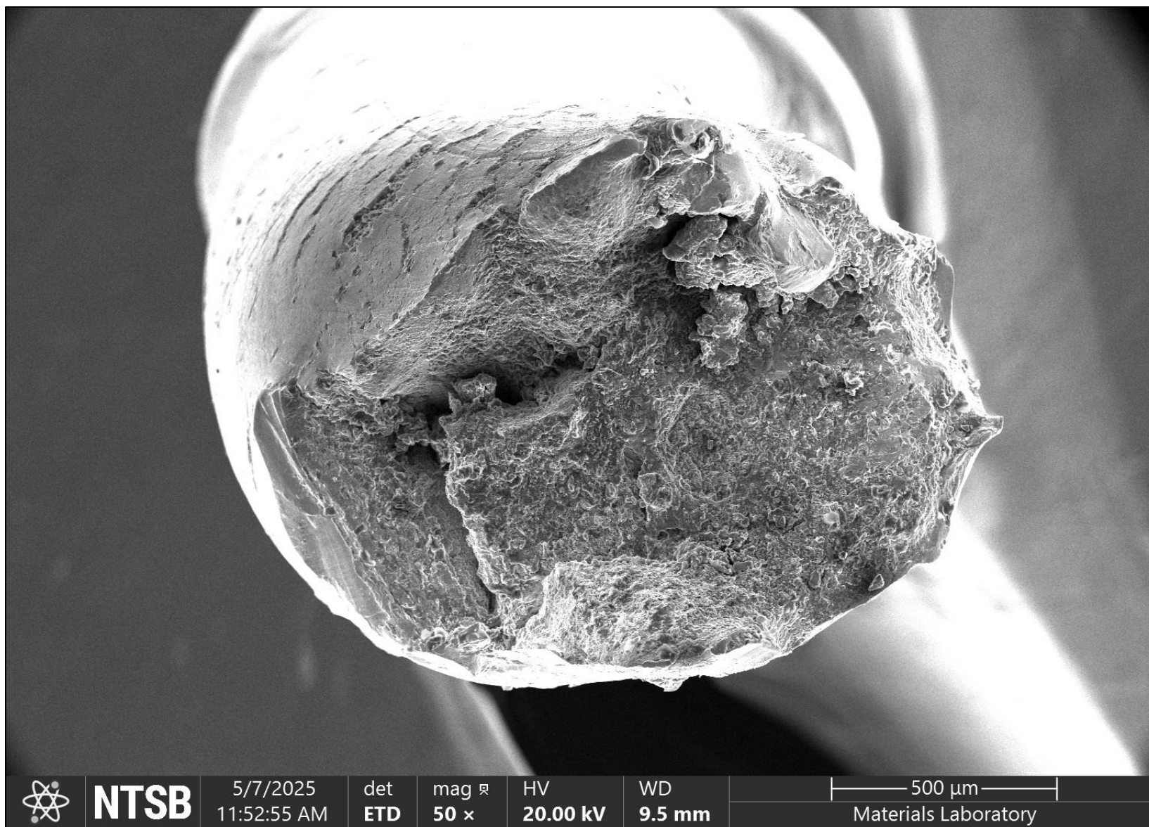
Photograph 2 - SEM of fracture surface. (50x)
