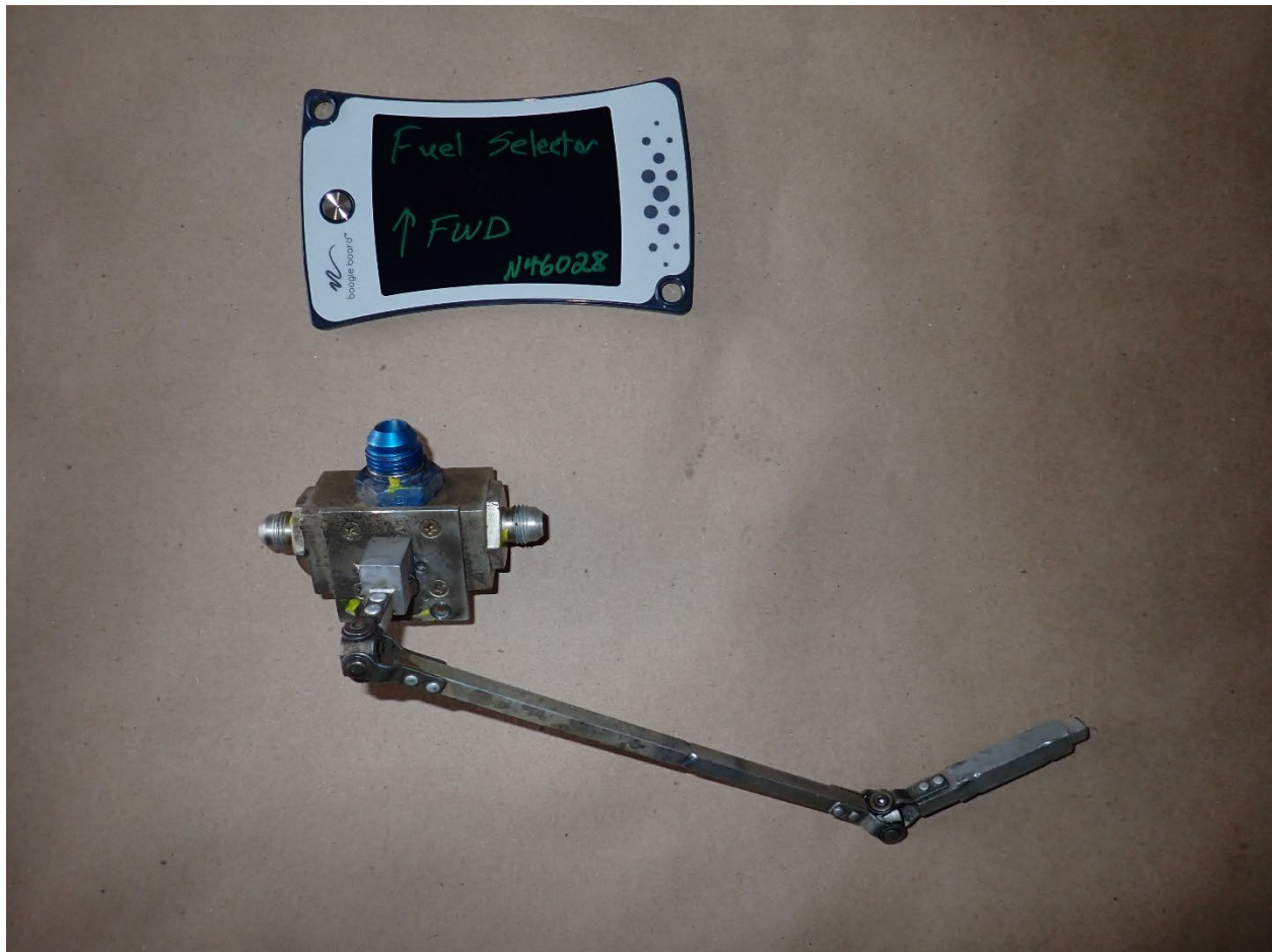
Figure 6: View of the fuel selector removed from the airframe for examination and function test
