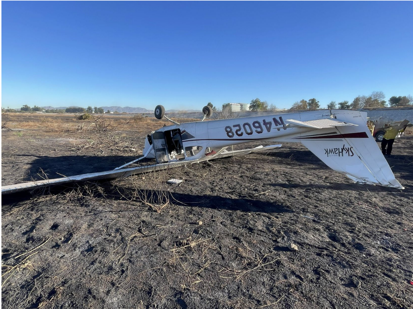
Photograph 3 - View of inverted airplane with damage to vertical stabilizer and rudder (Courtesy of FAA)
