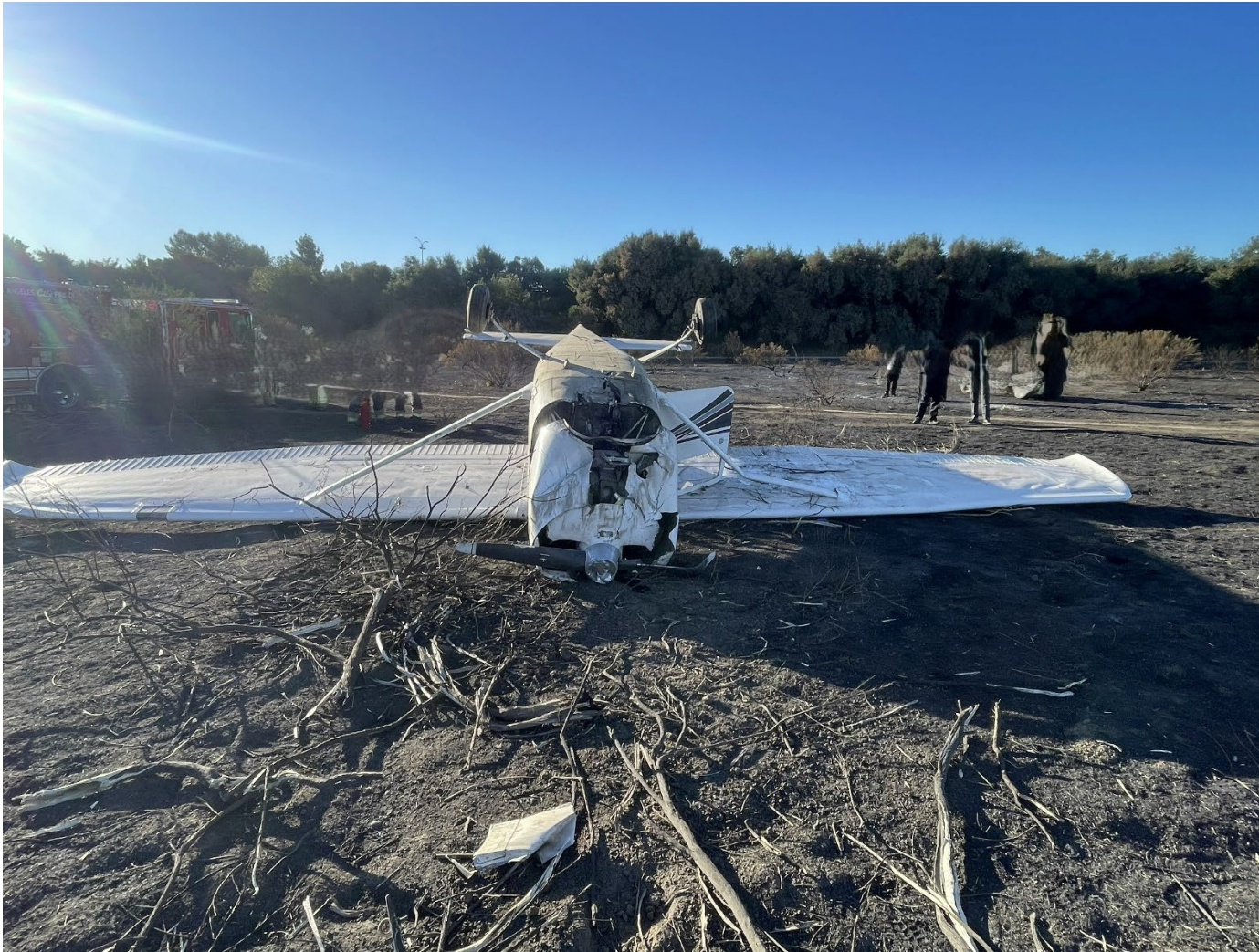
Photograph 2 - Forward to aft view of inverted airplane with substantial damage to right wing lift strut (Courtesy of FAA)
