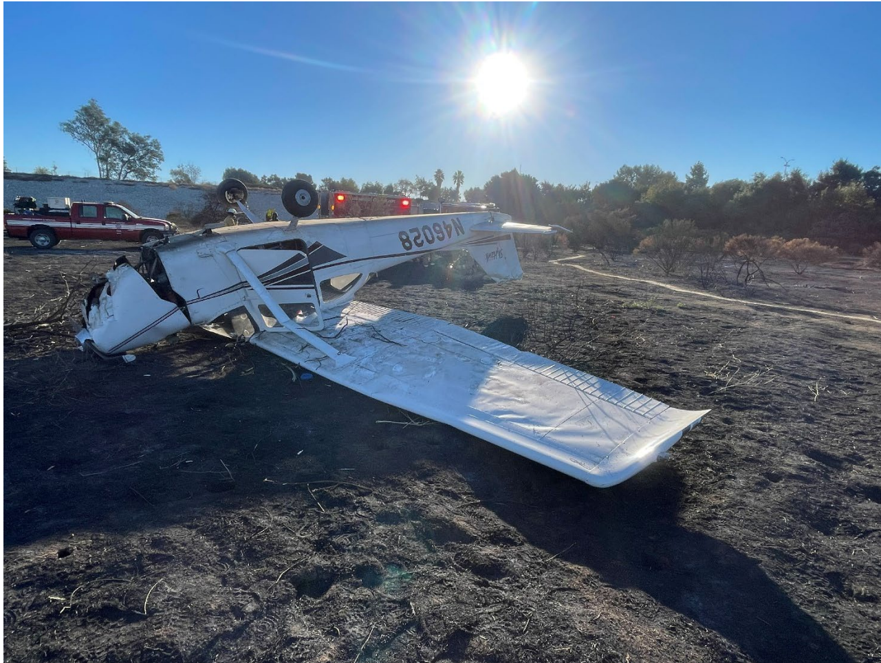
Photograph 1 - View of inverted airplane and substantial damage to the right wing lift strut, vertical stabilizer and rudder (Courtesy of FAA)
