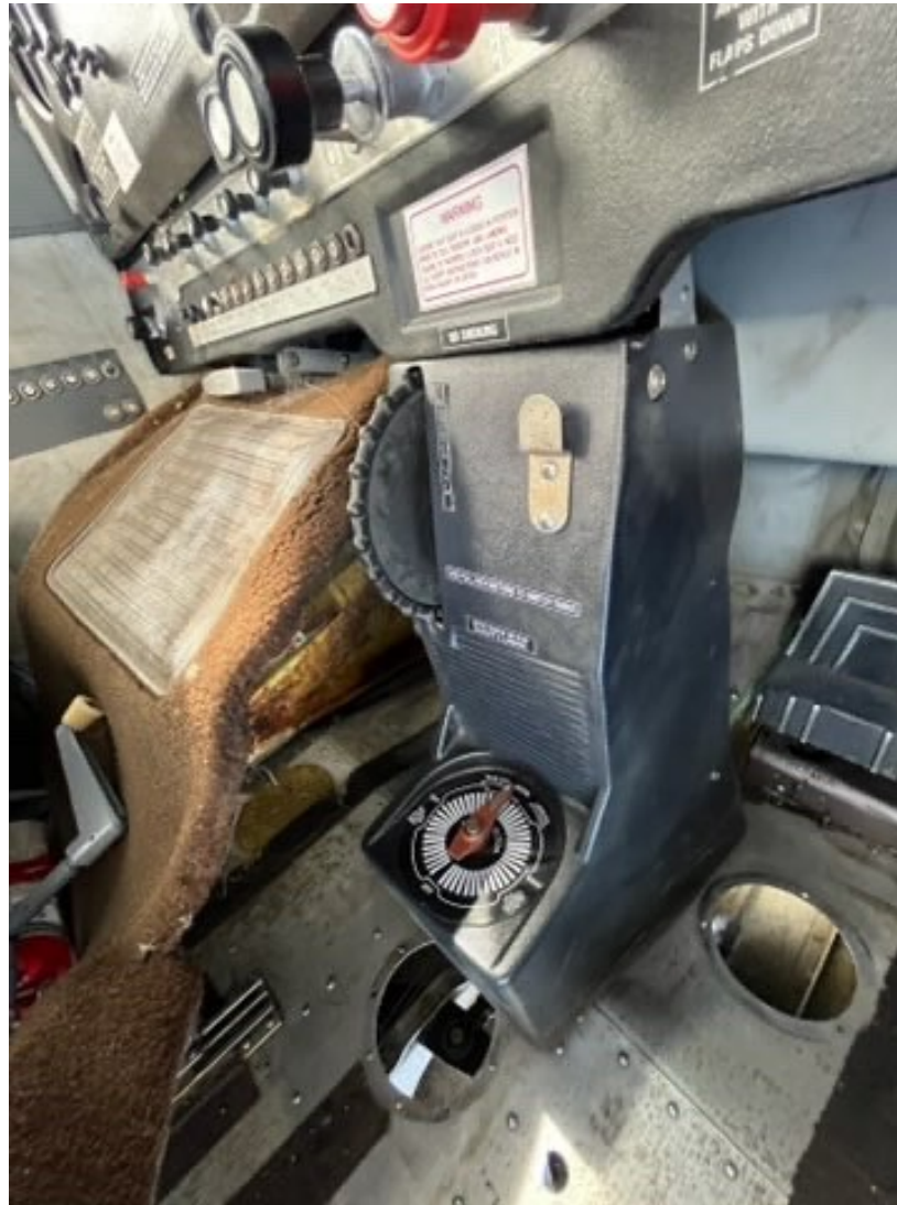
Photograph 4 - Onsite view of the airplane's fuel selector in the Both position (Courtesy of FAA)
