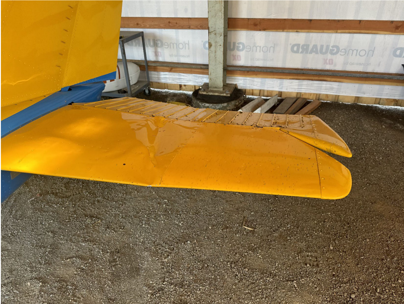
Photograph 2 - View of left horizontal Stabilizer damage (Courtesy of Pilot)
