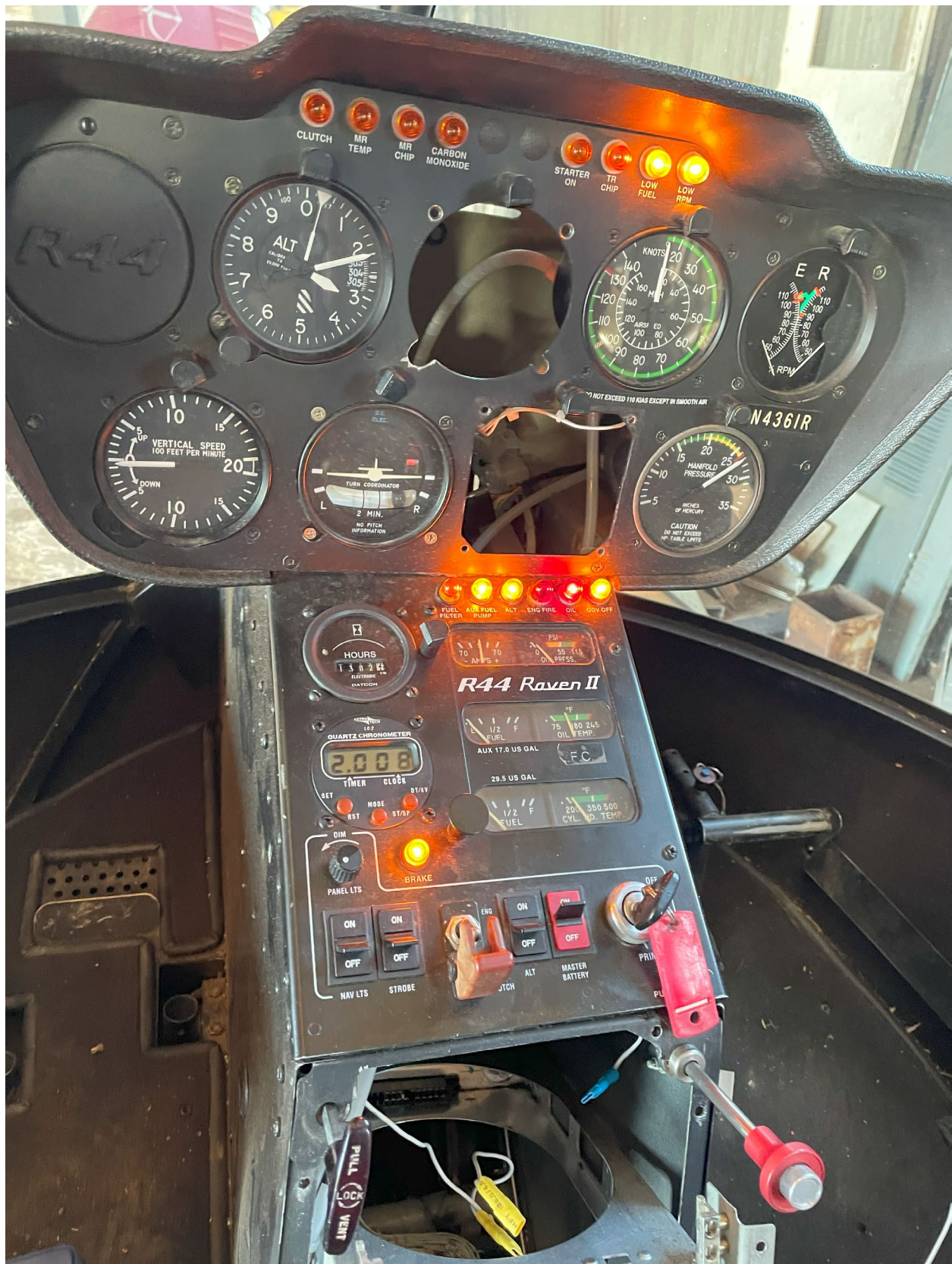
Figure 8. Instrument panel with power applied.
