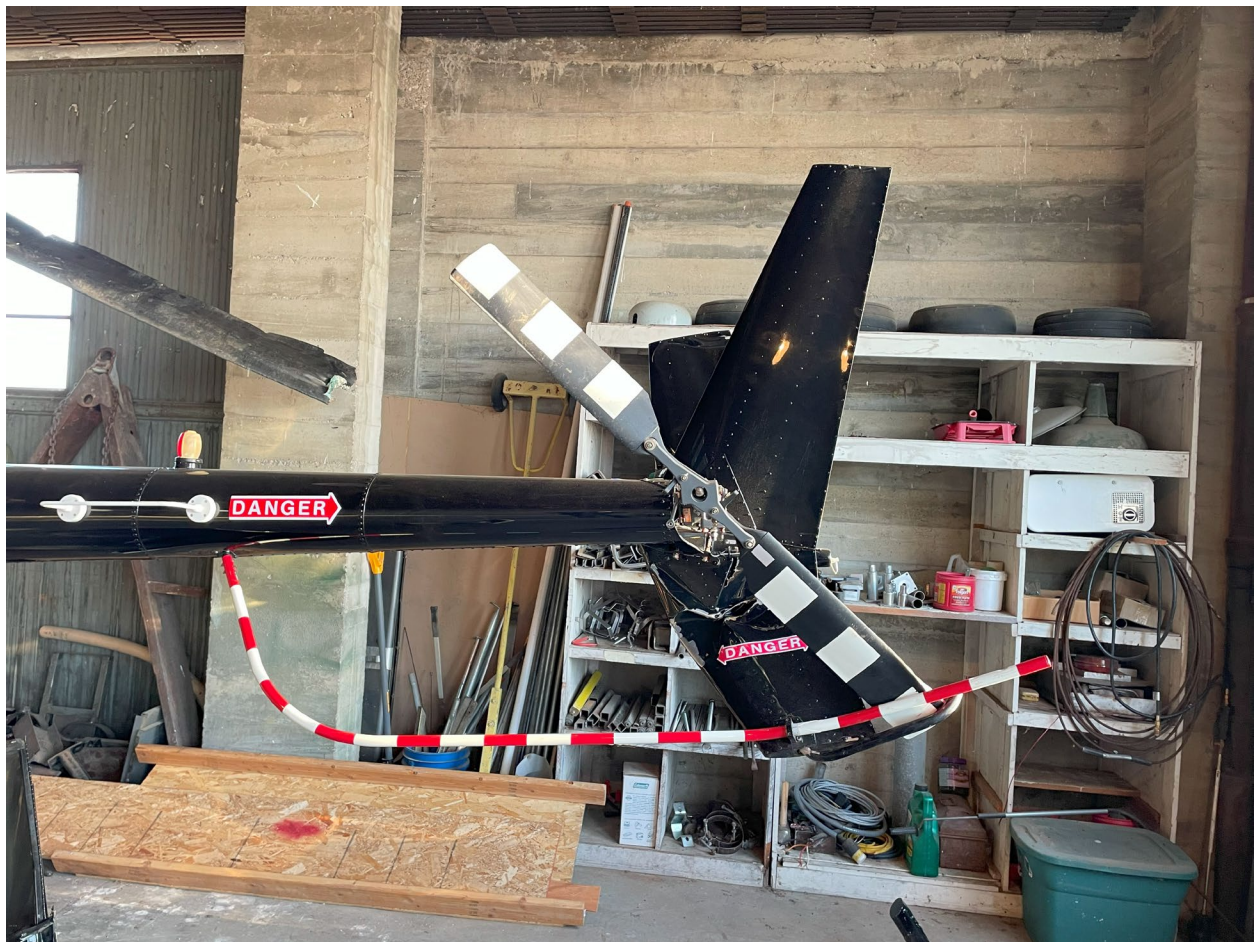
Figure 3. Tail rotor assembly, and Main rotor blade B.
