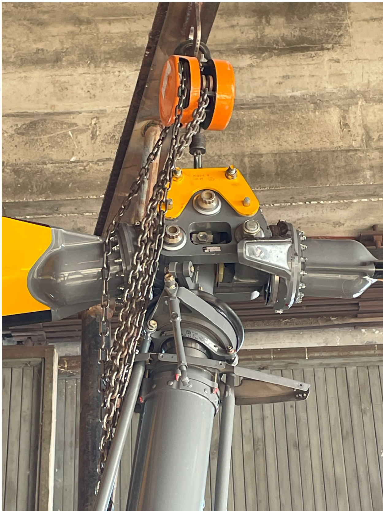
Figure 7. View of main rotor hub assembly and swashplate assembly.
