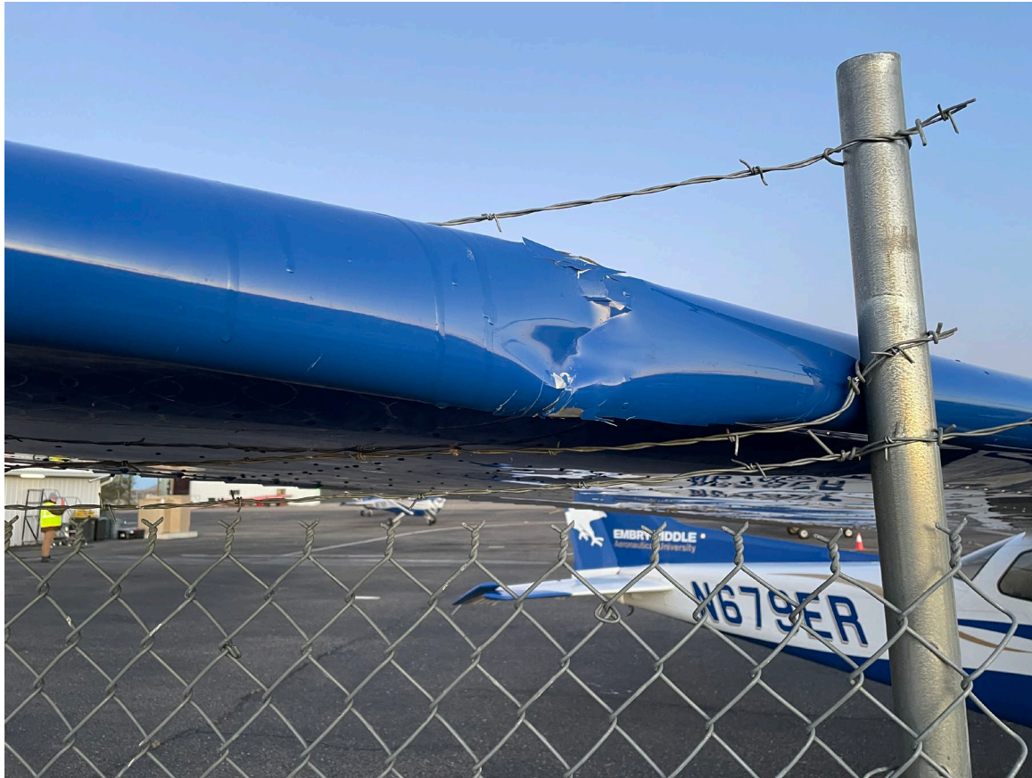
Photograph 1 - View of damage to right wing. (Courtesy of operator.)
