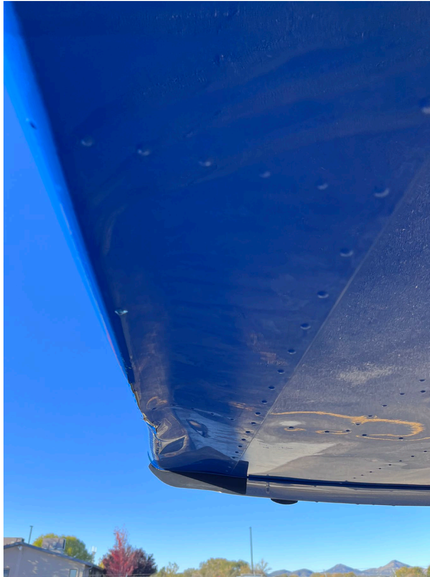
Photograph 2 - View of damage to right wing. (Courtesy of operator.)
