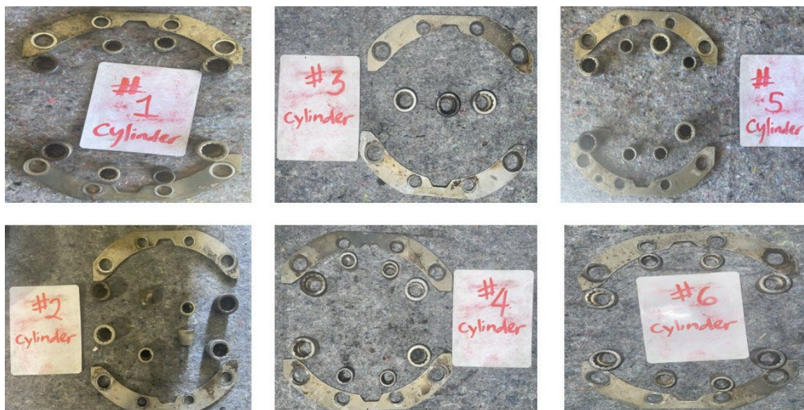
Photograph 6 - Photos showing fretting to each cylinder hold down plate (Courtesy of NTSB)
