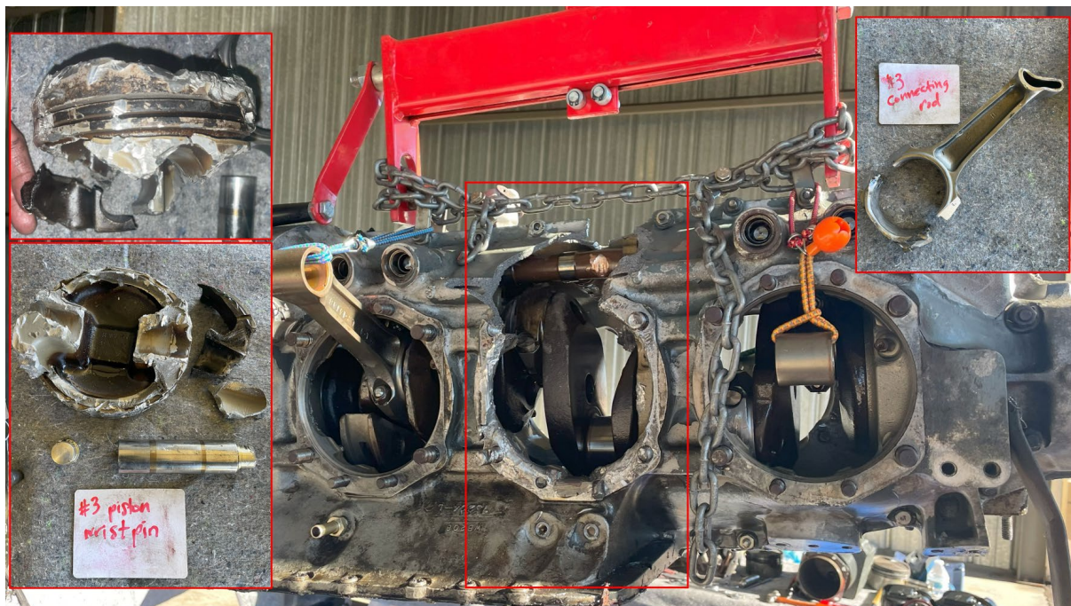
Figure 5. View of engine case highlighting damage to No. 3 cylinder mating surface and studs. Upper left and lower left photo: view of damage to No. 3 piston; Upper right photo: view of damaged connecting rod.
