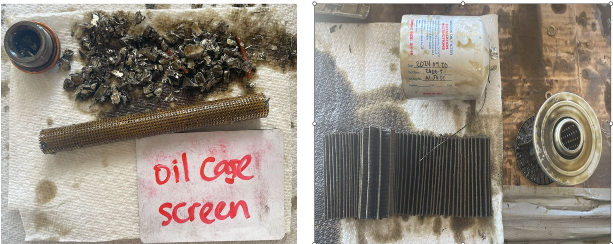
Figure 9. Left photo: view of oil case screen; right photo: view of removed oil filter.
