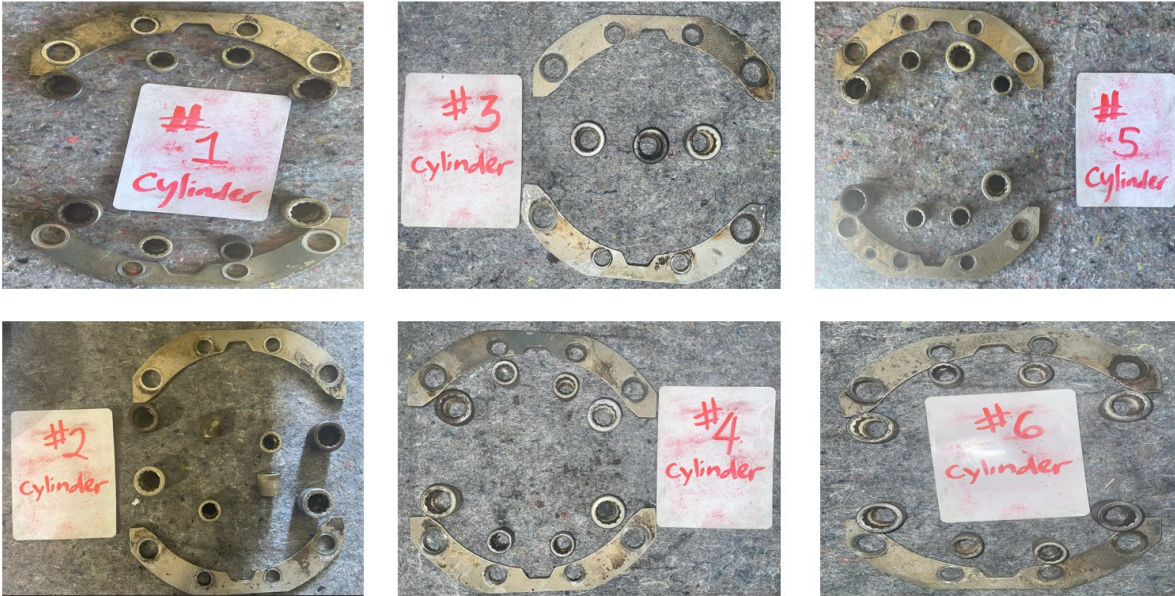
Figure 7. Six photos showing fretting to each cylinder hold down plate.
