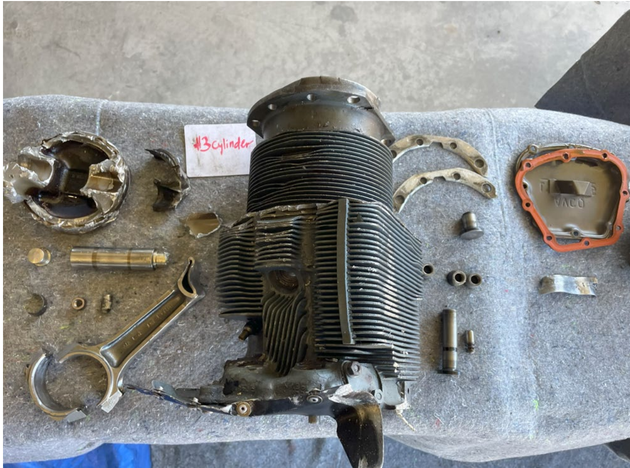
Figure 3. View of No. 3 cylinder and recovered parts.
