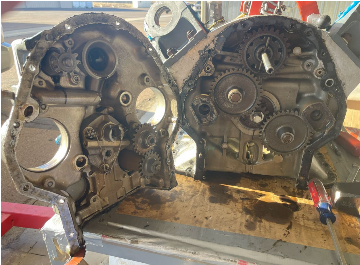
Figure 4. Internal view of accessory gearbox.
