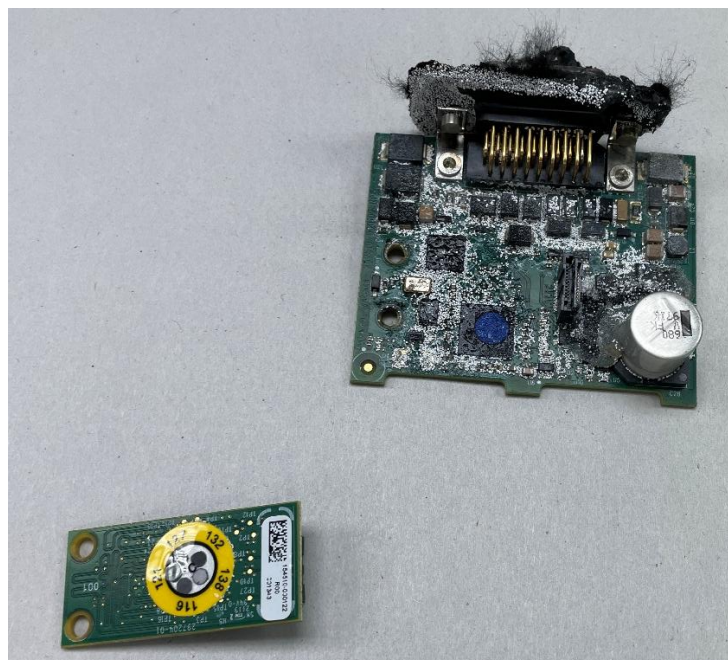
Figure 2. Memory module (bottom left) and main circuit board (top right).
