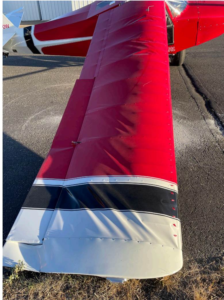
Photo 2 – Damage to right wing and right aileron (courtesy of Federal Aviation Administration)
