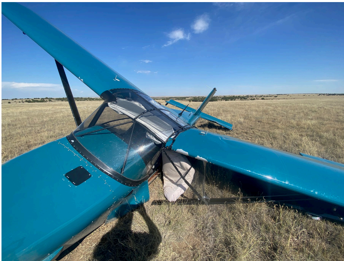
Photograph 1 - View of wing and tail damage (Courtesy of FAA)
