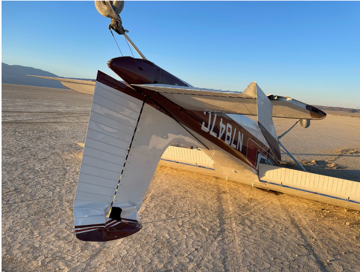
Photograph 3 - View of substantial damage to the empennage. (Courtesy of the pilot.)
