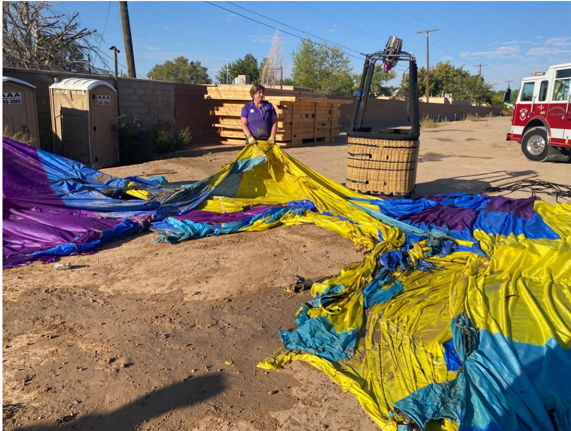
Photograph 1 - Accident site, envelope damage. (Courtesy of the FAA)
