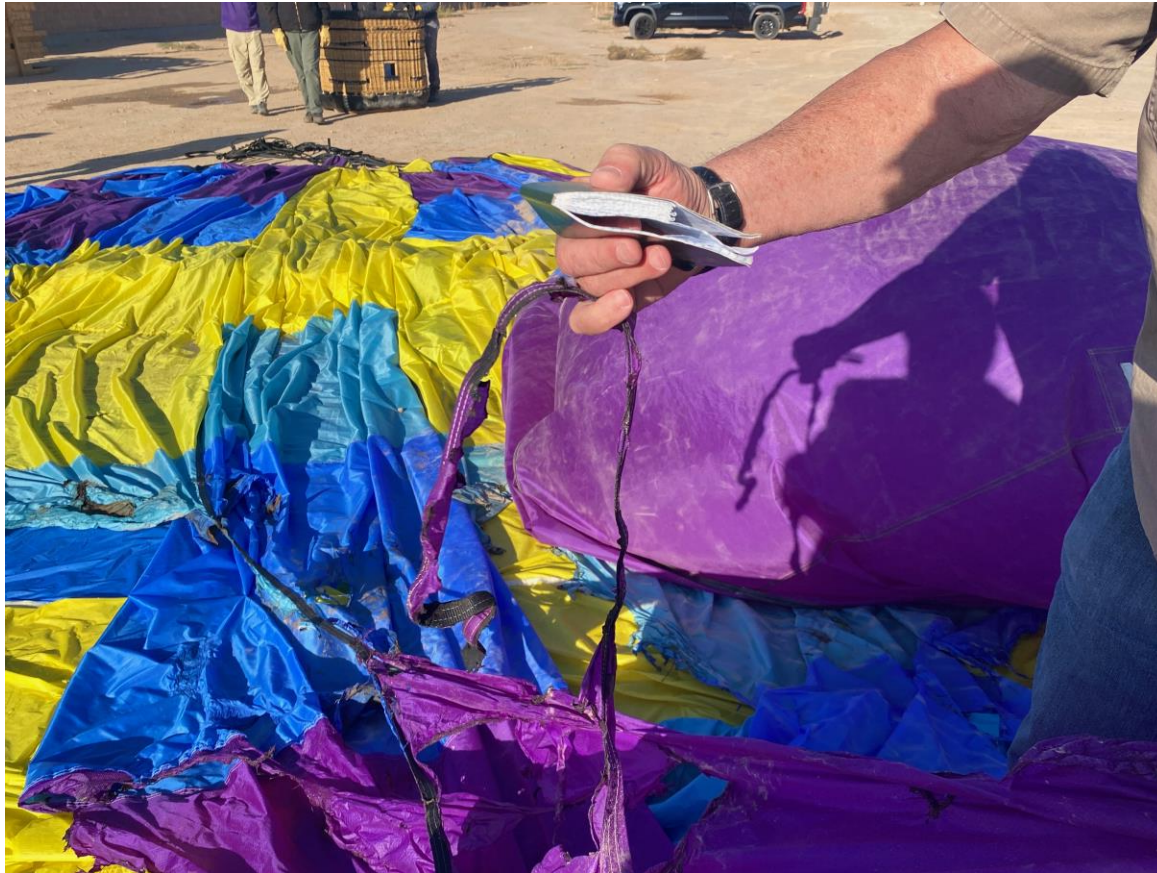
Photograph 3 - Accident site, envelope damage. (Courtesy of the FAA)
