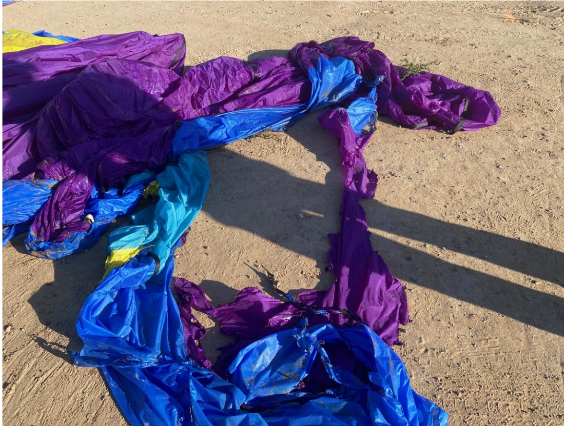
Photograph 2 - Accident site, envelope damage. (Courtesy of the FAA)
