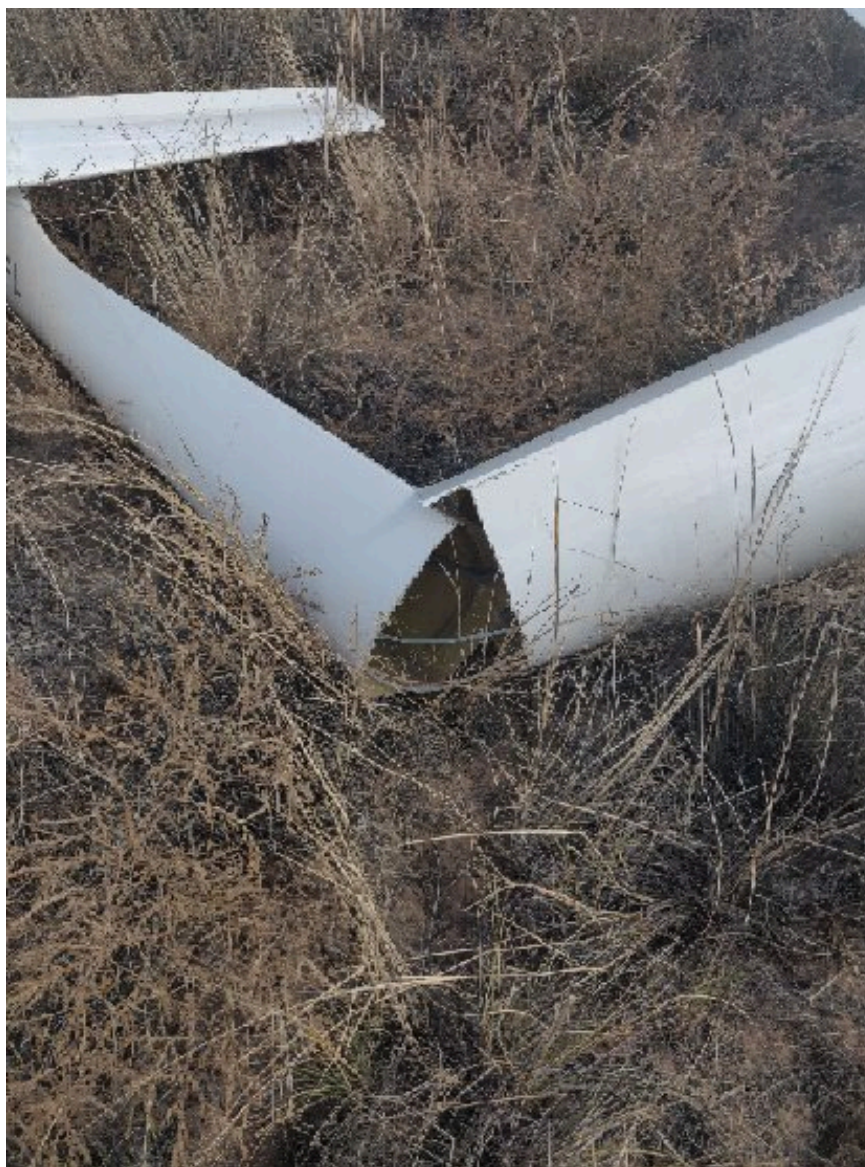
Photograph 3 - View of substantial damage to empennage. (Courtesy of airport operations.)
