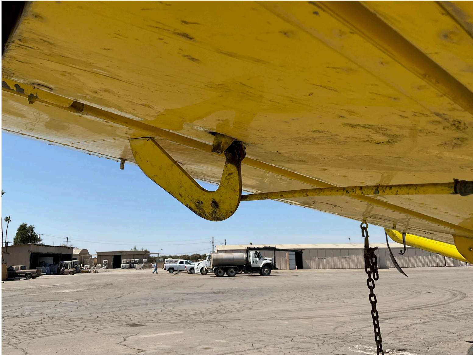
Photograph 3 - Damaged aileron hinge and boost tab control rod (Courtesy of FAA)
