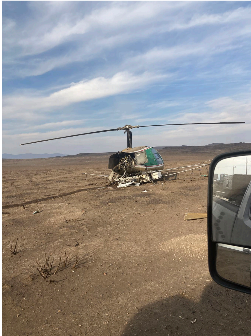
Photograph 1 - View of damage to helicopter tailboom (Courtesy of the pilot)
