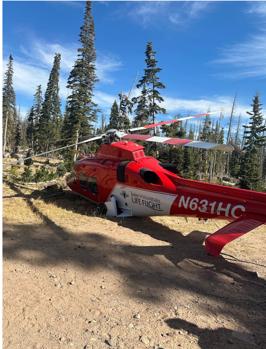
Photograph 1 - View of damage to the helicopter's left main landing gear strut and lower fuselage (Courtesy of operator)
