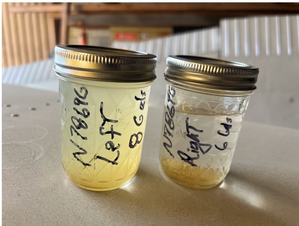
Photograph 3 - Left- and right-wing fuel samples showing contamination (Courtesy of Recovery agent)
