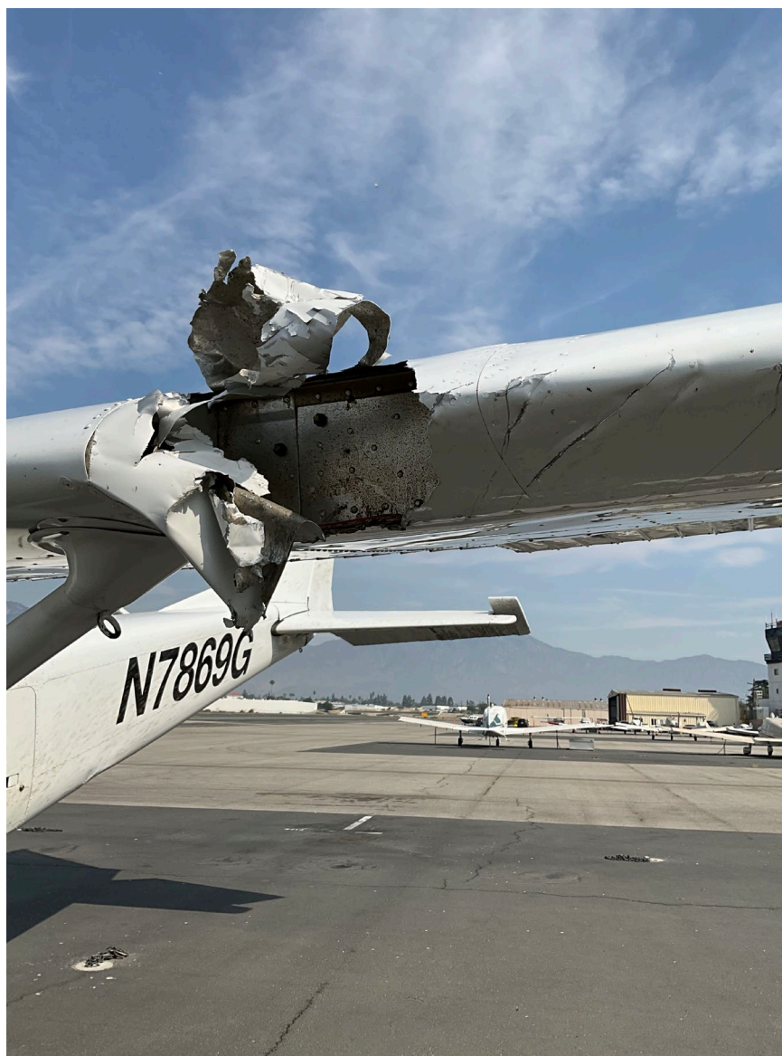
Photograph 2 - Substantial damage to the left-wing spar (Courtesy of airport manager)
