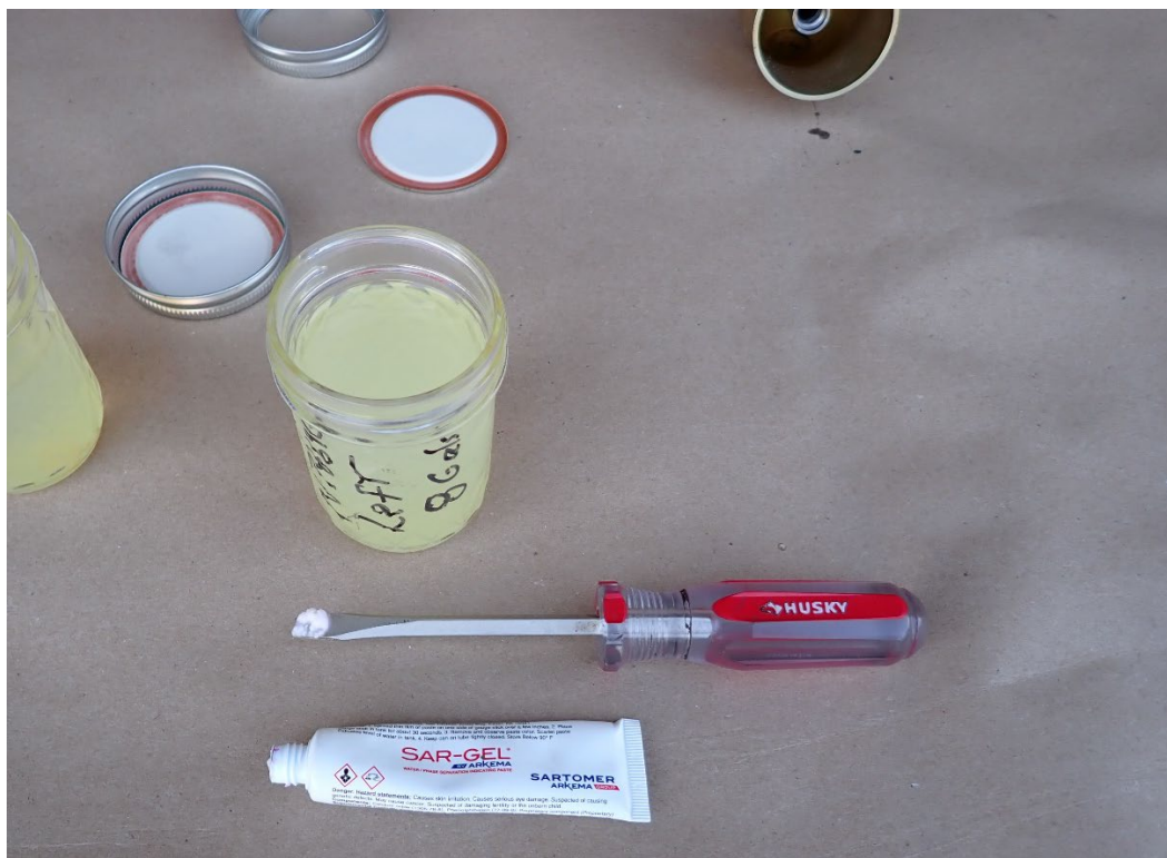
Figure 4: View of the left wing fuel sample water test.
