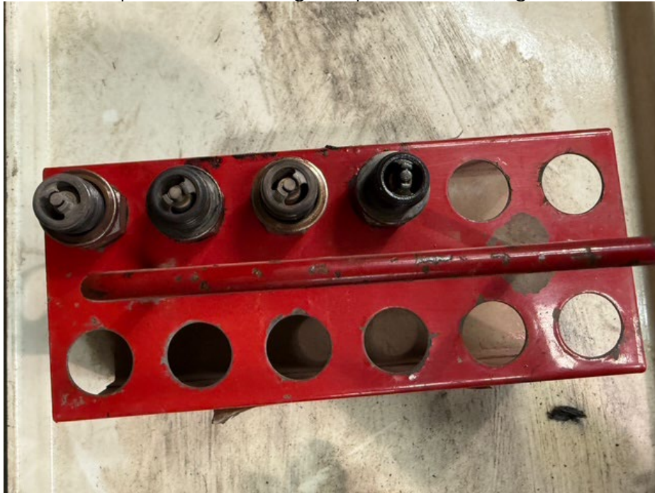
Figure 2 Top spark plugs from each cylinder
