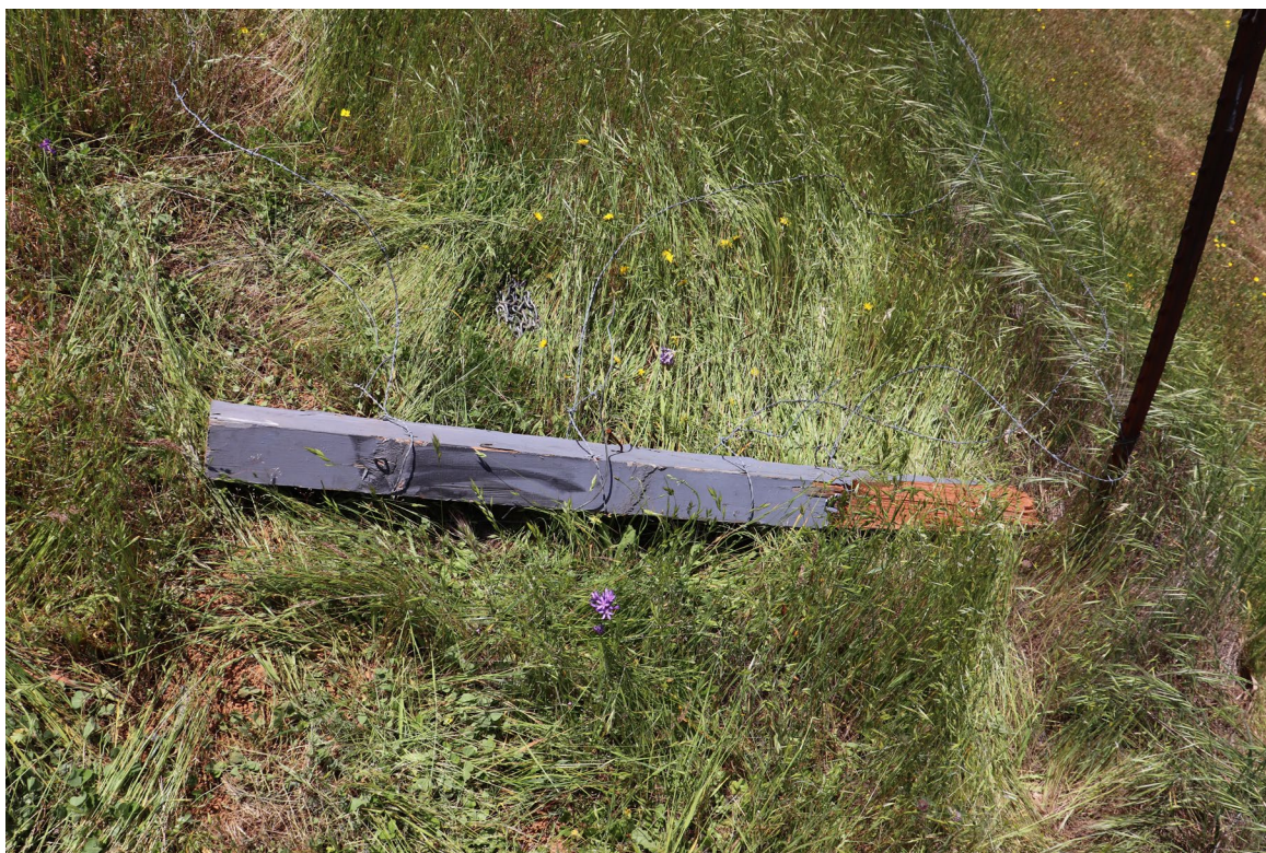
Photograph 4 - View of downed airport perimeter fence post with black transfer mark.
