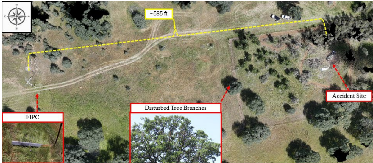
Figure 3: Screenshot of point cloud generated by Pix4D depicting areas of interest.
