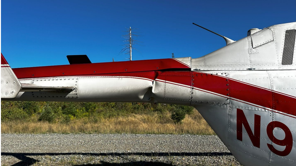
Figure 3. Tailboom downward buckle near boom station 42.59. [Source: JL Aviation]
