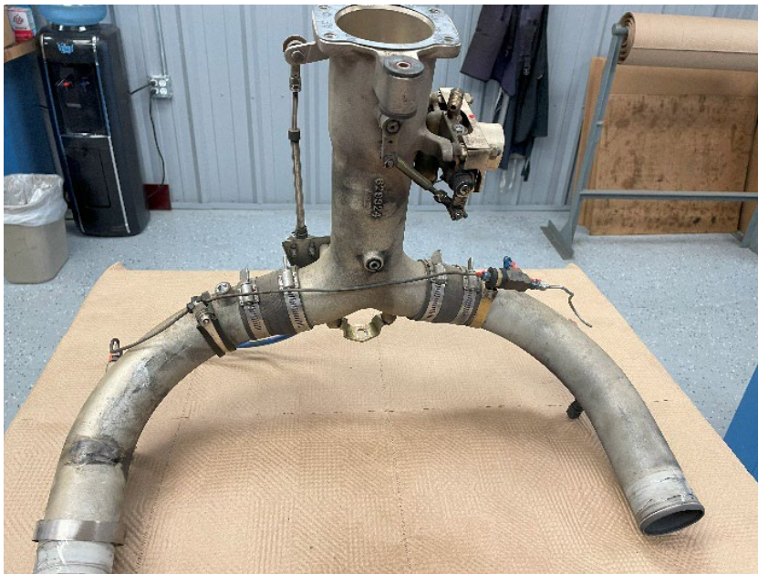
Figure 7. View of throttle body.
