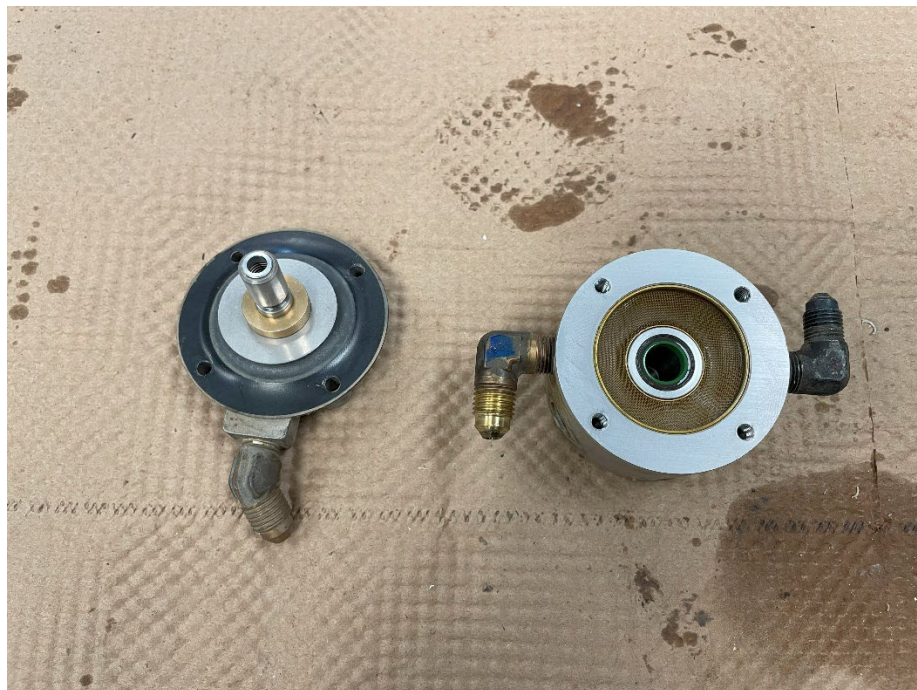
Figure 11. View of disassembled fuel manifold.
