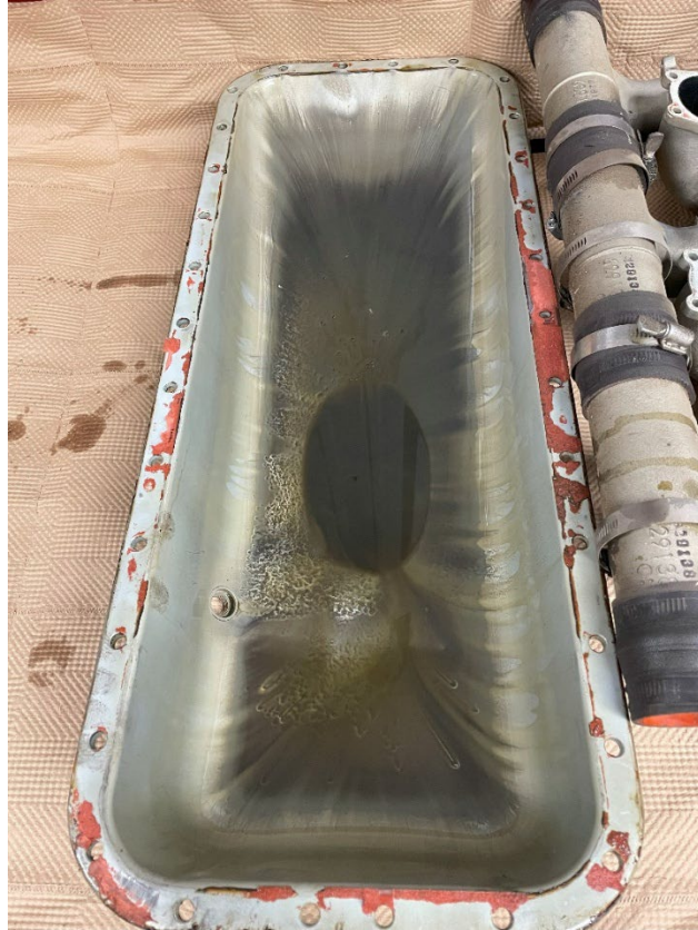
Figure 12. View of the oil sump.
