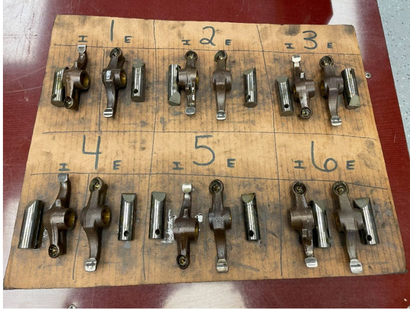
Figure 13. View of rocker arms and push rods.
