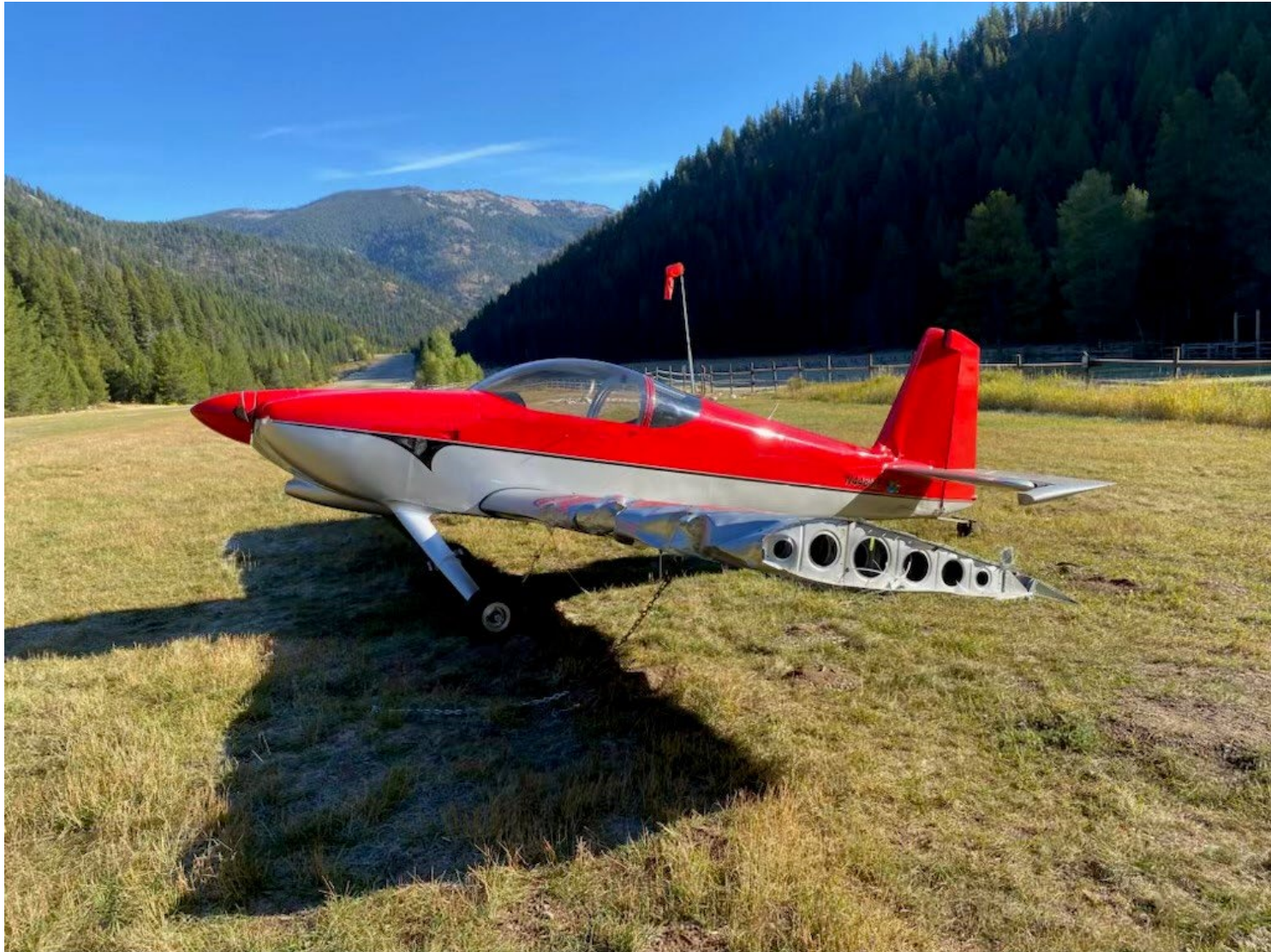
Photograph 1 - View of left wing and tail damage (Courtesy of pilot)
