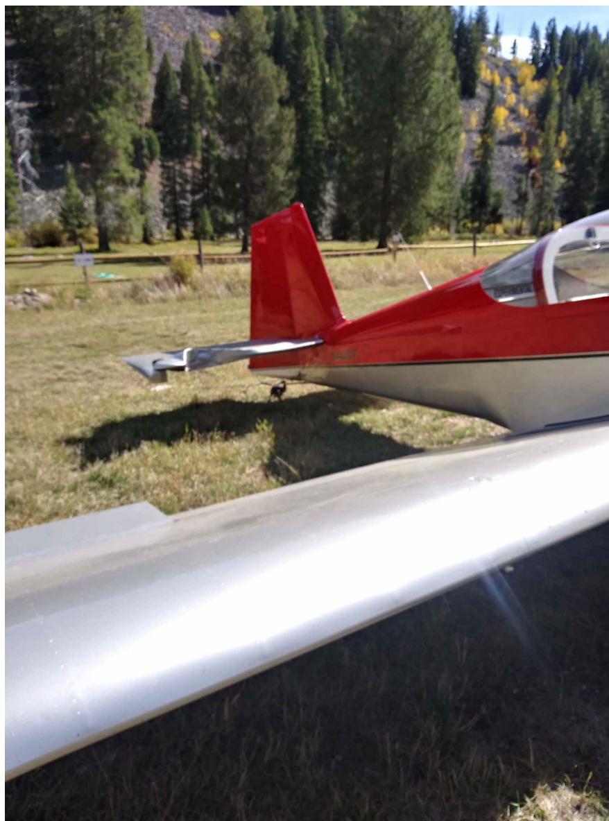
Photograph 2 - View of right horizontal stabilizer damage (Courtesy of pilot)
