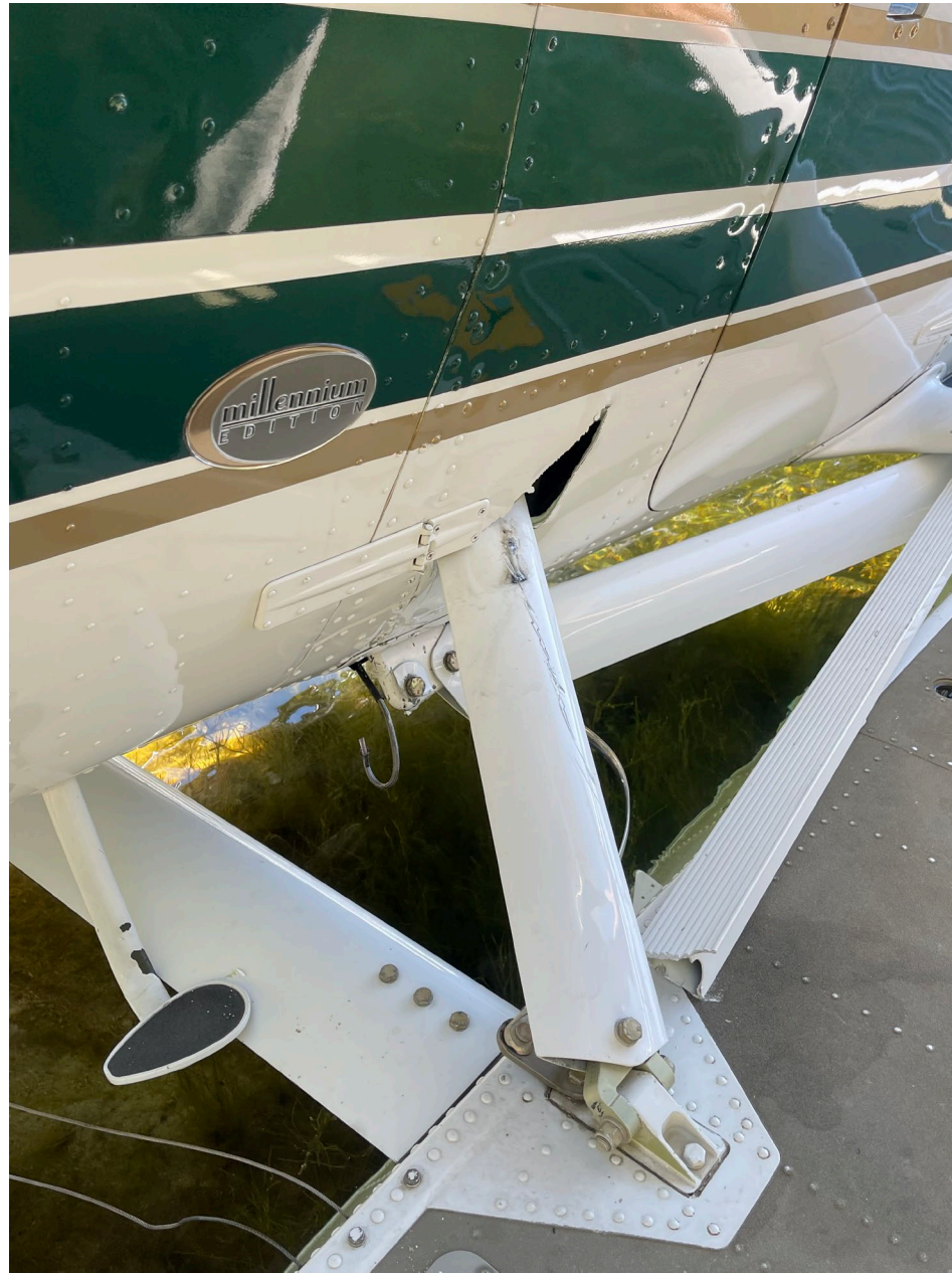
Photo 1 – View of damage to fuselage (courtesy of wreckage recovery)
