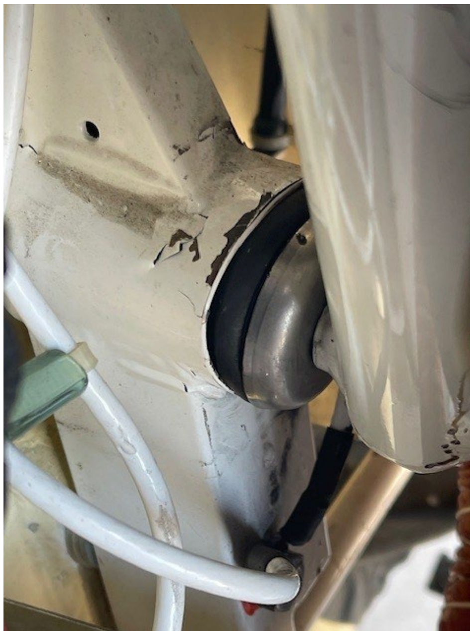
Photo 3 – Substantial damage to mount. Source owner.
