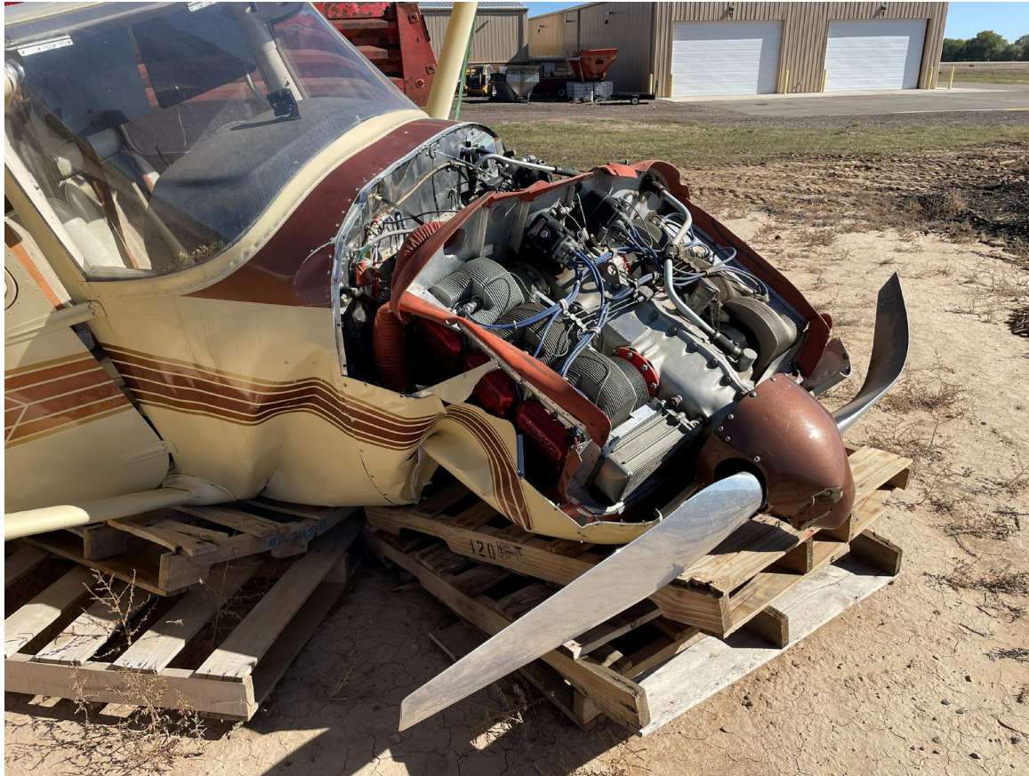
Photograph 2 - View of damaged right lower fuselage and engine compartment
