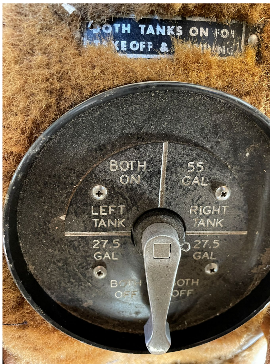
Photograph 6 - View of fuel selector and caption "Both tanks on for takeoff and landing."
