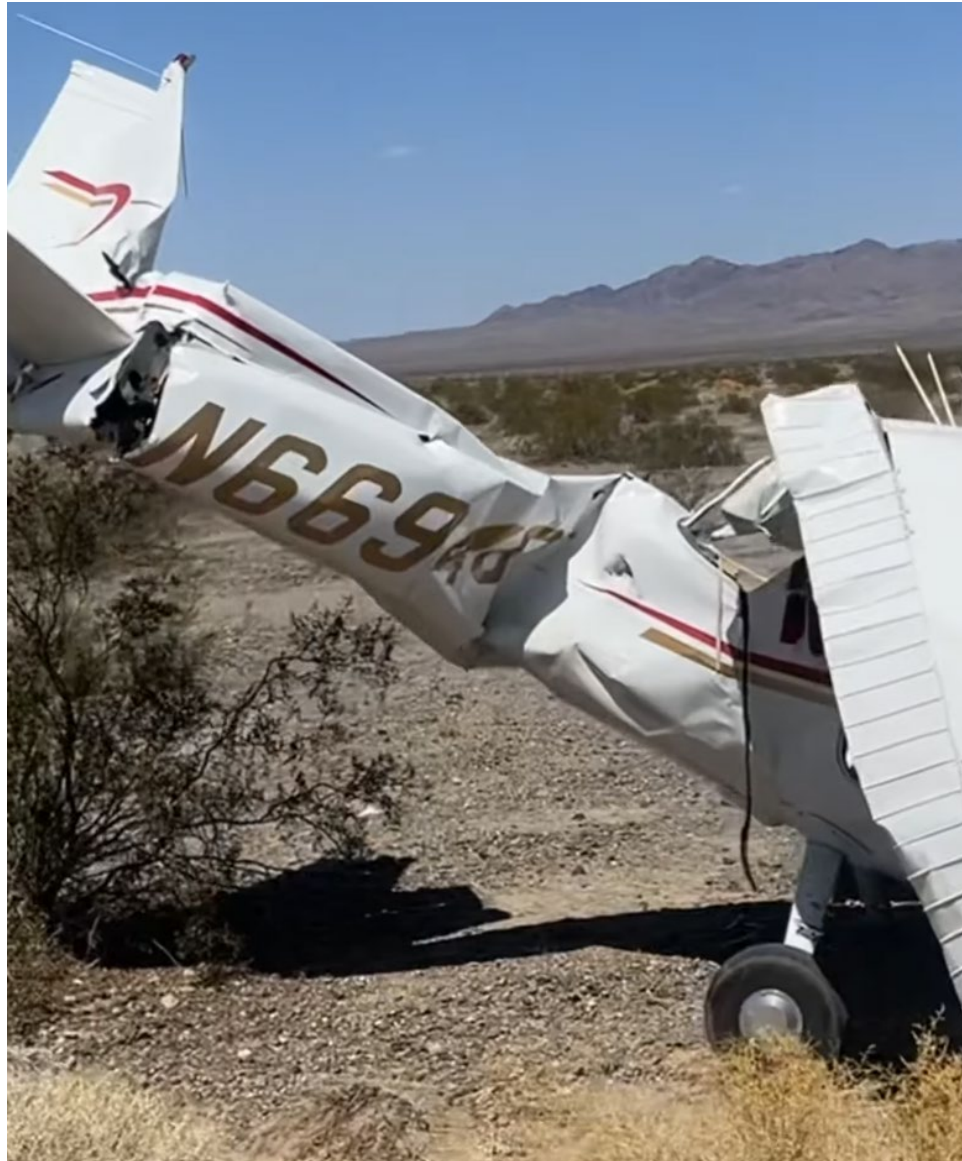
Photograph 1 - View of damaged aft fuselage (Courtesy of law enforcement officer)
