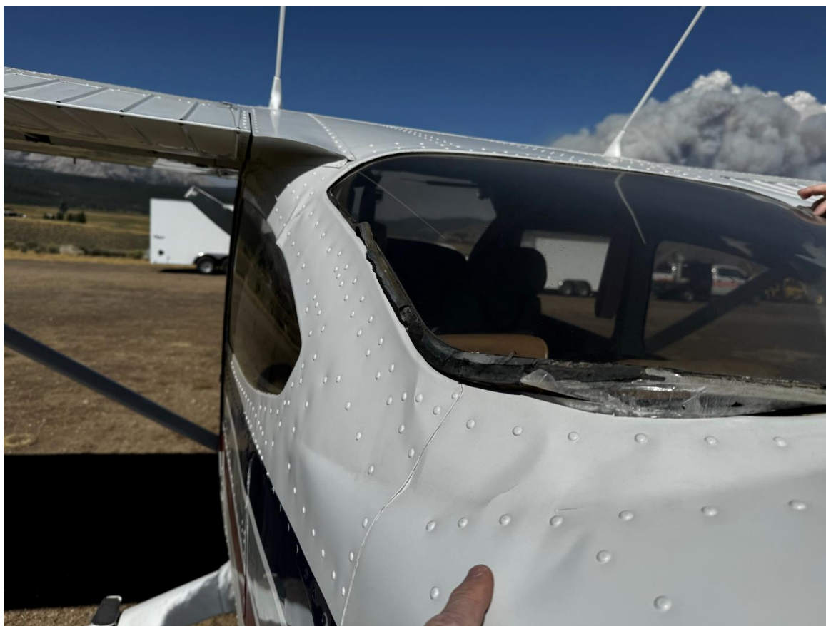
Photograph 6 - Airplane aft fuselage damage. (Courtesy of the pilot.)
