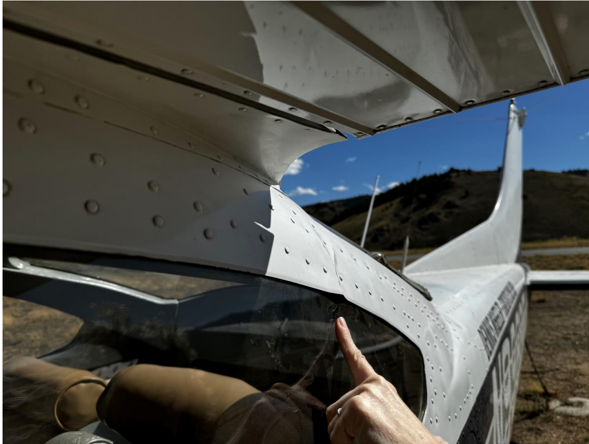
Photograph 5 - Airplane aft fuselage damage. (Courtesy of the pilot.)
