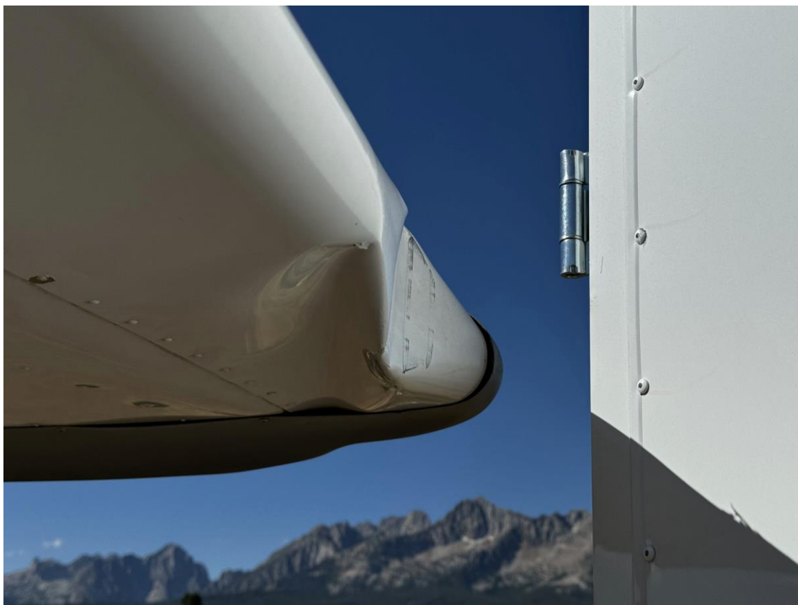
Photograph 1 - Left wing impact damage and parked trailer. (Courtesy of the pilot.)
