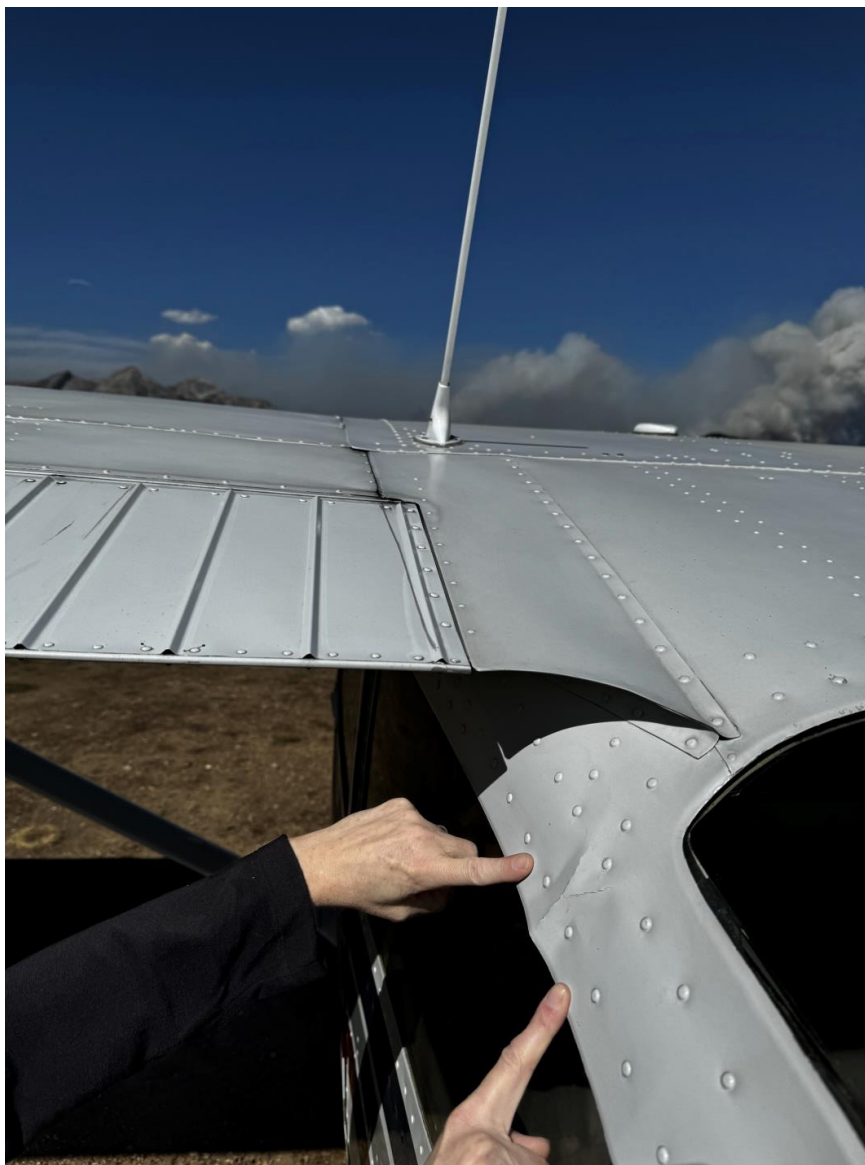
Photograph 4 - Airplane aft fuselage damage. (Courtesy of the pilot.)
