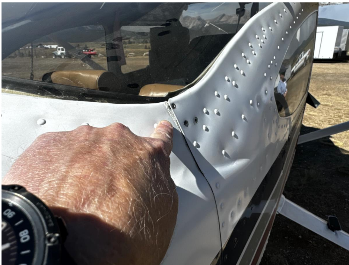
Photograph 3 - Airplane aft fuselage damage. (Courtesy of the pilot.)
