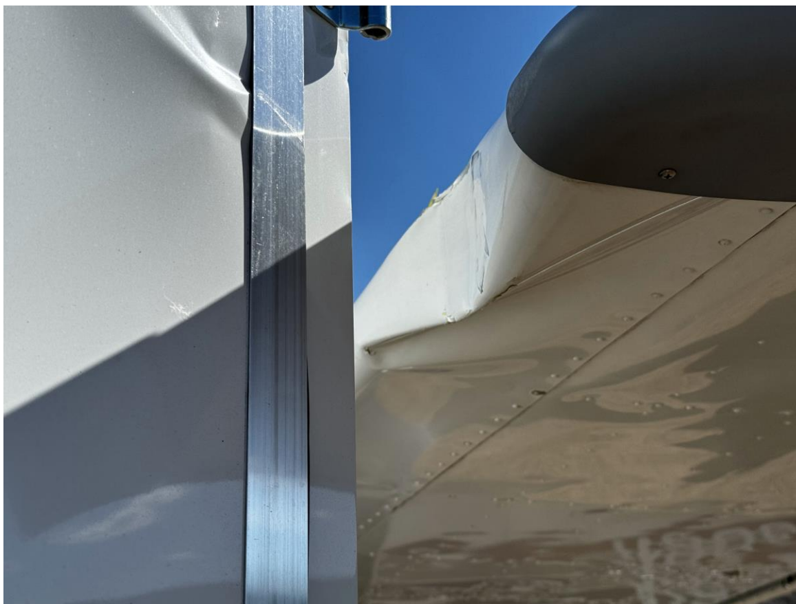
Photograph 2 - Left wing damage and parked trailer. (Courtesy of the pilot.)
