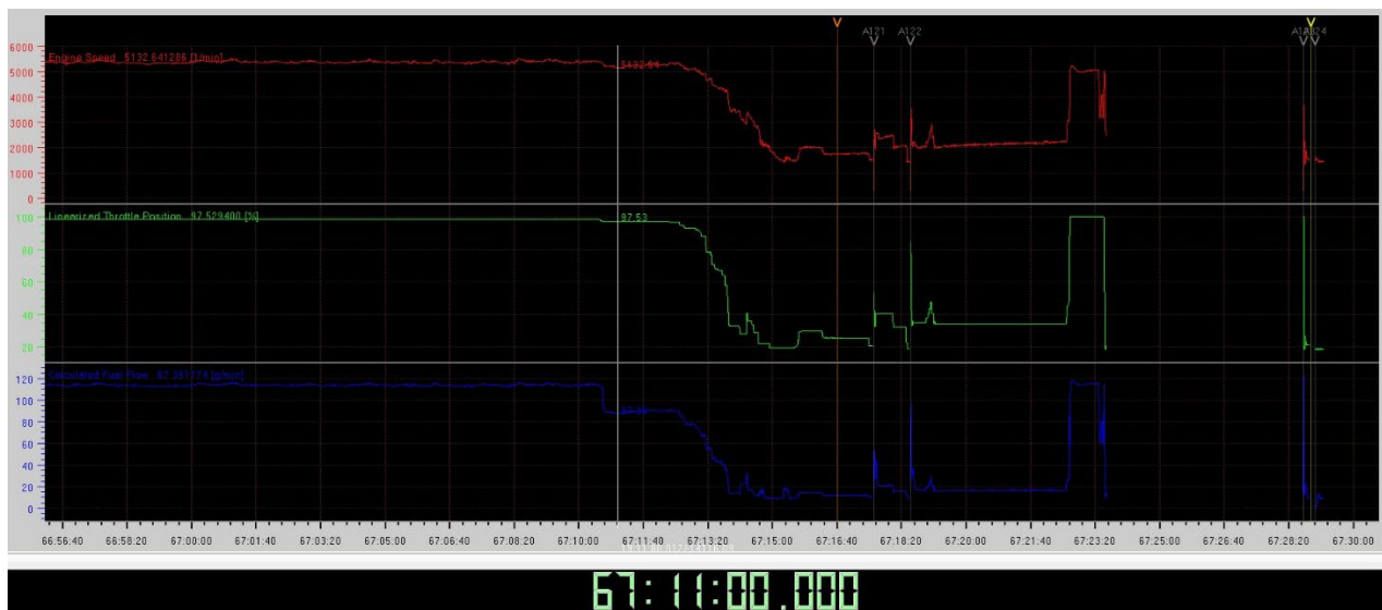
Figure 3: Accident flight Engine Speed, Linearized Throttle Position, and Calculated Fuel Flow parameters.
