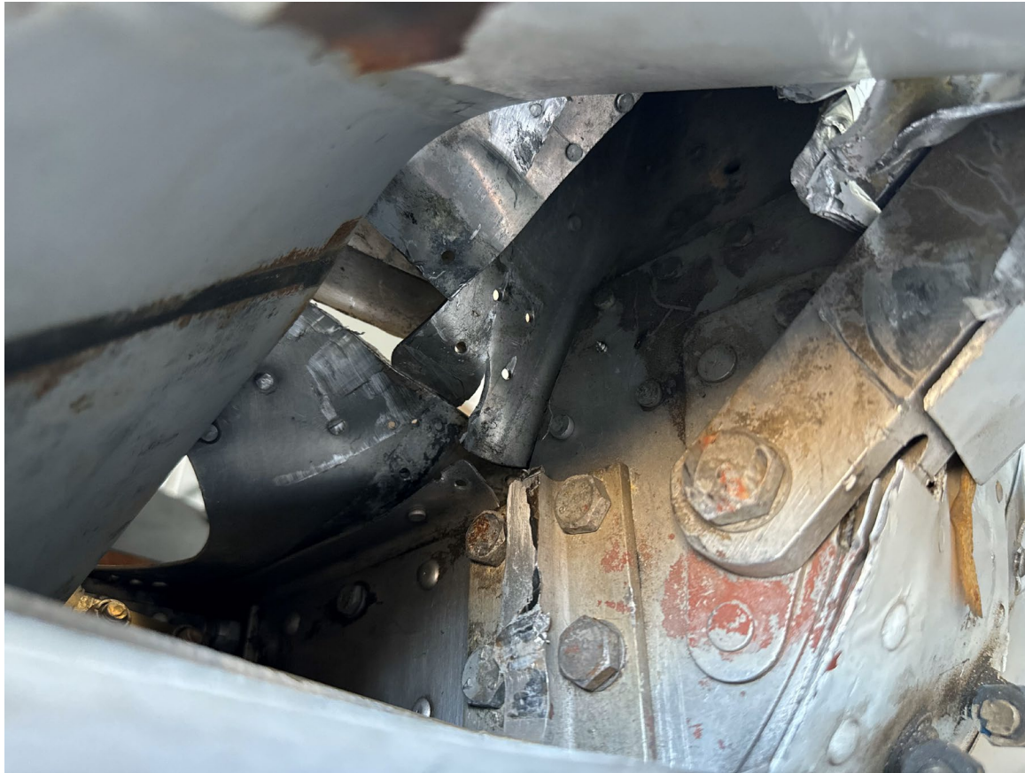
Photograph 3 - View of substantial damage to fuselage structure. (Courtesy of pilot.)
