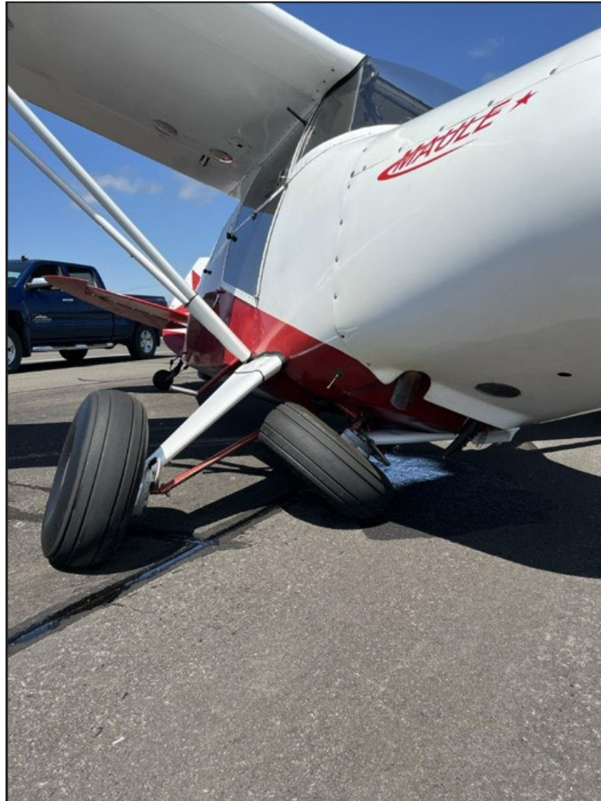
Photograph 3 - Main Gear Collapse (Courtesy of Pilot)
