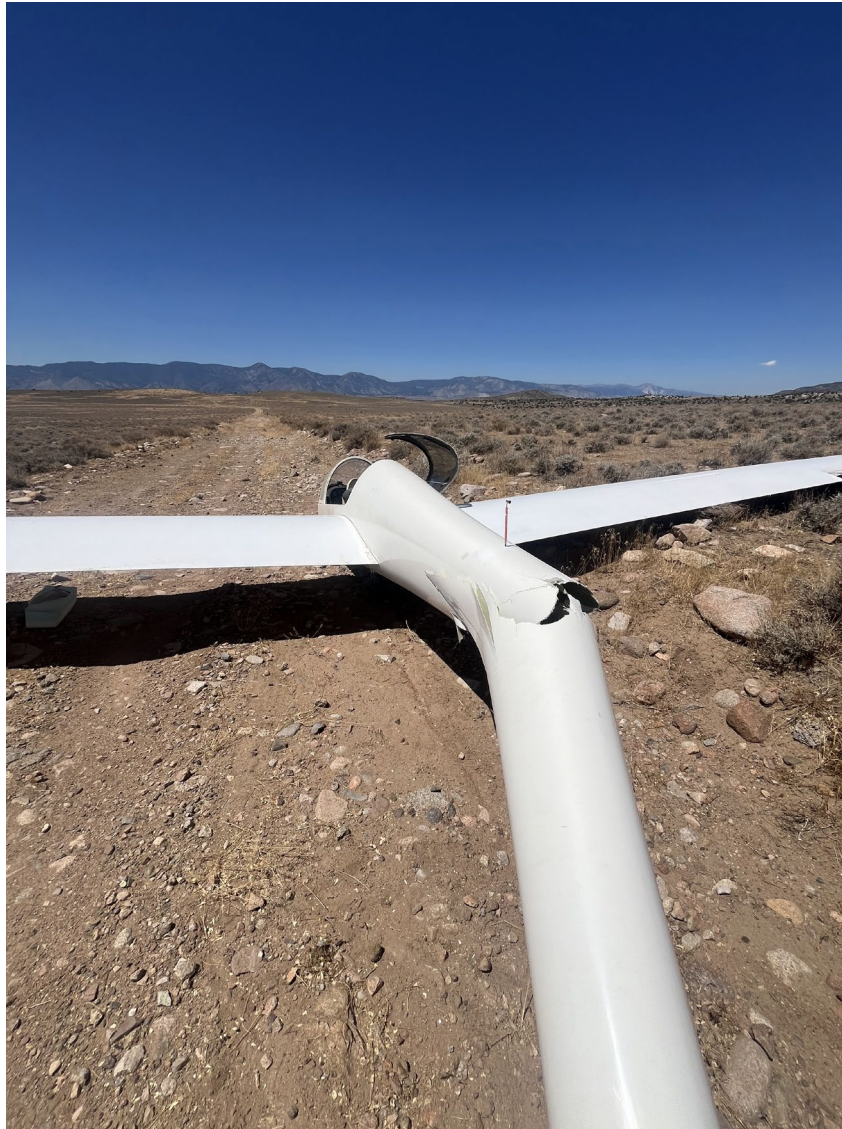
Photograph 2 - Sailplane tailcone damage (courtesy of pilot)
