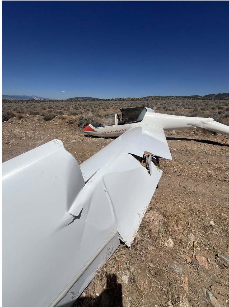
Photograph 1 - Sailplane left wing damage (courtesy of pilot)
