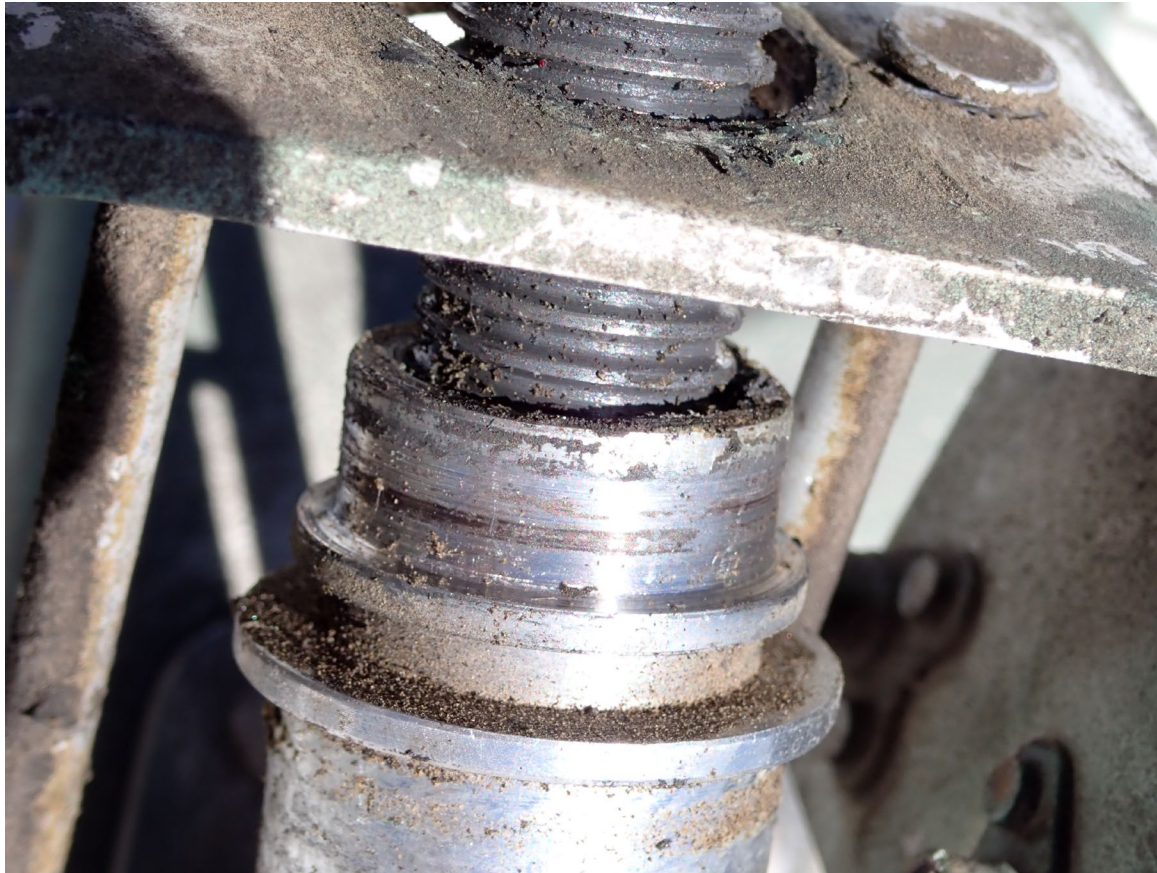
Photograph 3 - View of stabilator trim screw assembly
