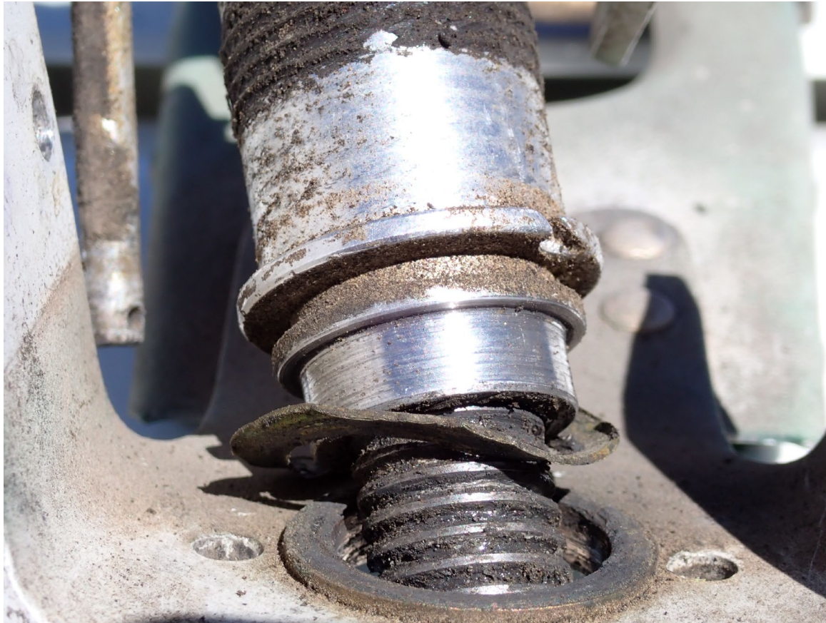
Photograph 4 - View of stabilator trim screw assembly
