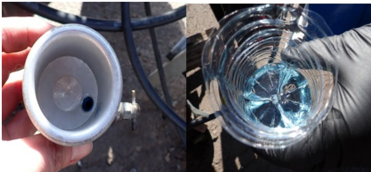
Figure 7. Left photo: view of removed gascolator; right photo: view of recovered fuel from gascolator. Photo courtesy of Continental Aerospace Technologies.
