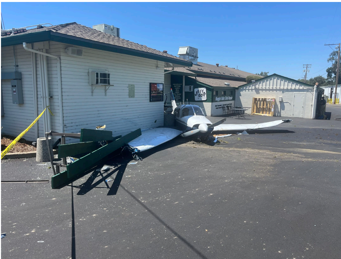
Photograph 2 - View of accident airplane adjacent a building with damage to both wings (Courtesy of the FAA)
