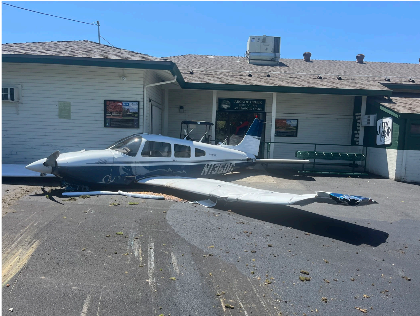
Photograph 1 - View of accident airplane with left wing and fuselage damage (Courtesy of the FAA)
