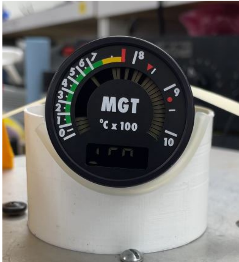
Figure 4 - Random screen characters as supply voltage drops below 6v
