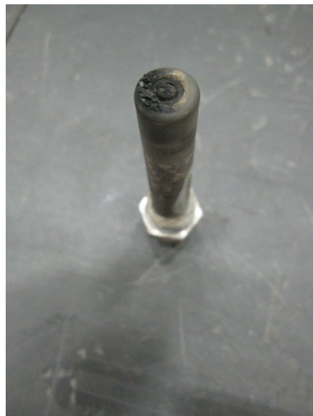
PHOTO 14: COKE BUILD-UP ON IGNITER PLUG
