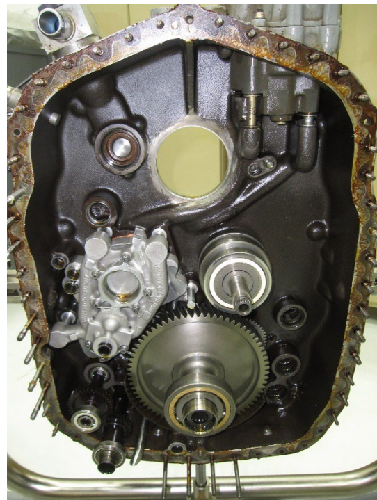
PHOTO 28: GP DRIVEN GEAR TRAIN IN ACCESSORY GEARBOX HOUSING
