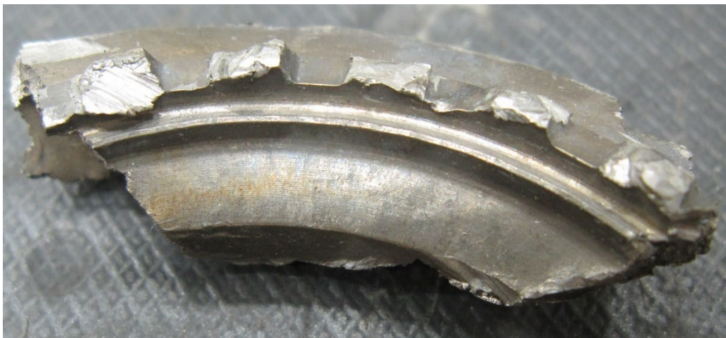
PHOTO 11: RECOVERED FRAGMENT OF CURVIC COUPLING TEETH
