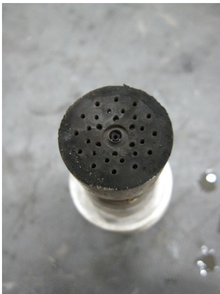
PHOTO 13: COKE BUILD-UP ON FUEL NOZZLE TIP
