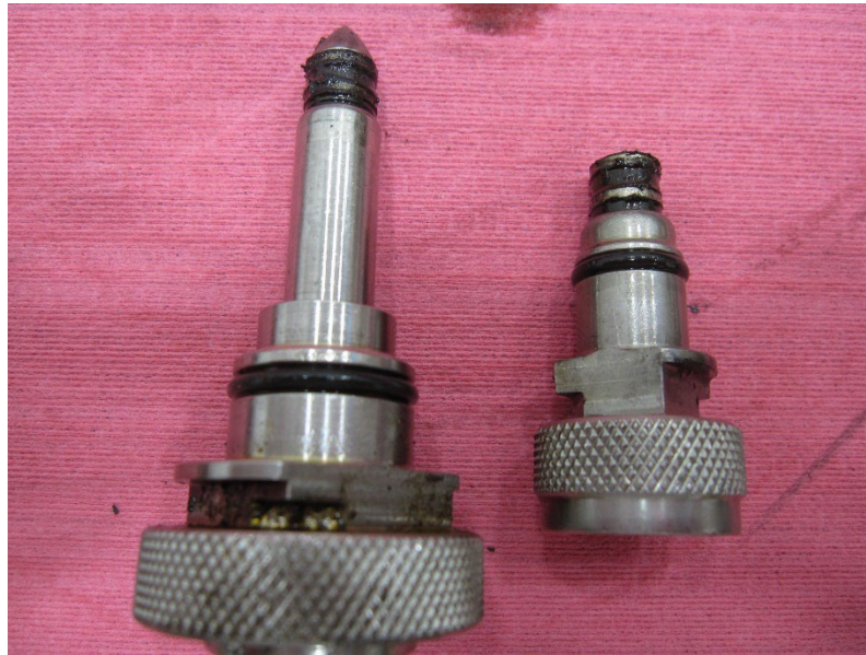
PHOTO 31: MAGNETIC CHIP DETECTORS FROM THE ACCESSORY GEARBOX HOUSING
