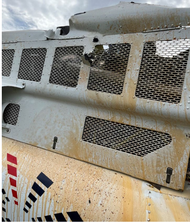
PHOTO 4: HELICOPTER FUSELAGE, RIGHT SIDE, COVERED IN OIL - WRECKAGE SITE
