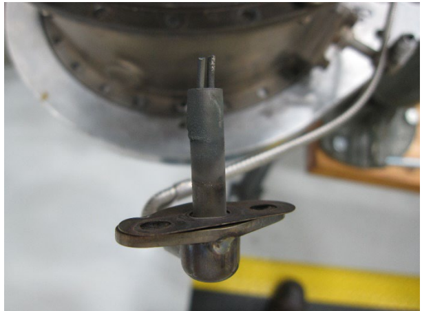
PHOTO 21: FRACTURED THERMOCOUPLE PROBE
