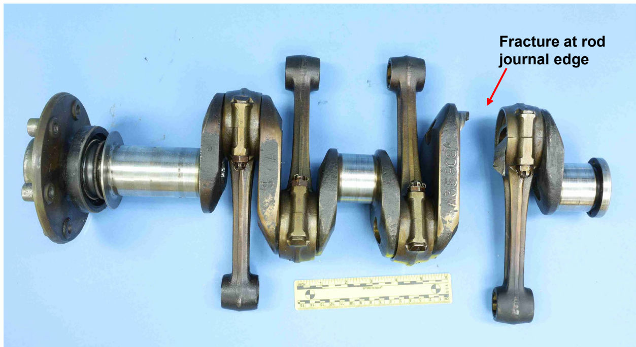
Figure 1. As-received overall crankshaft showing separation at the connecting rod journal.
