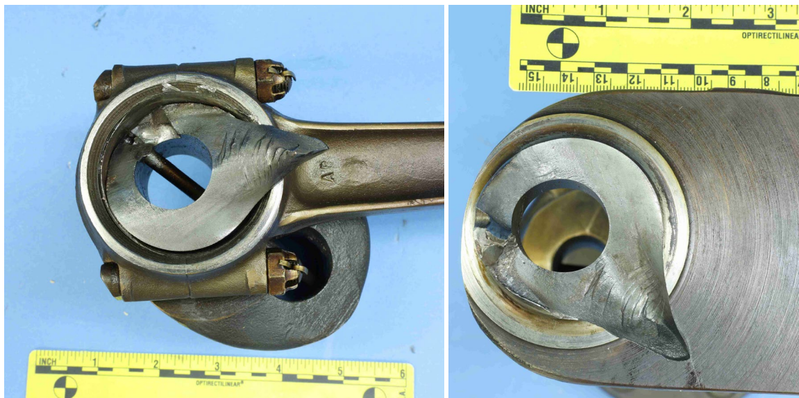
Figure 2. As-received images of the journal fracture surfaces at journal edge (left image) and at the web (right image).
