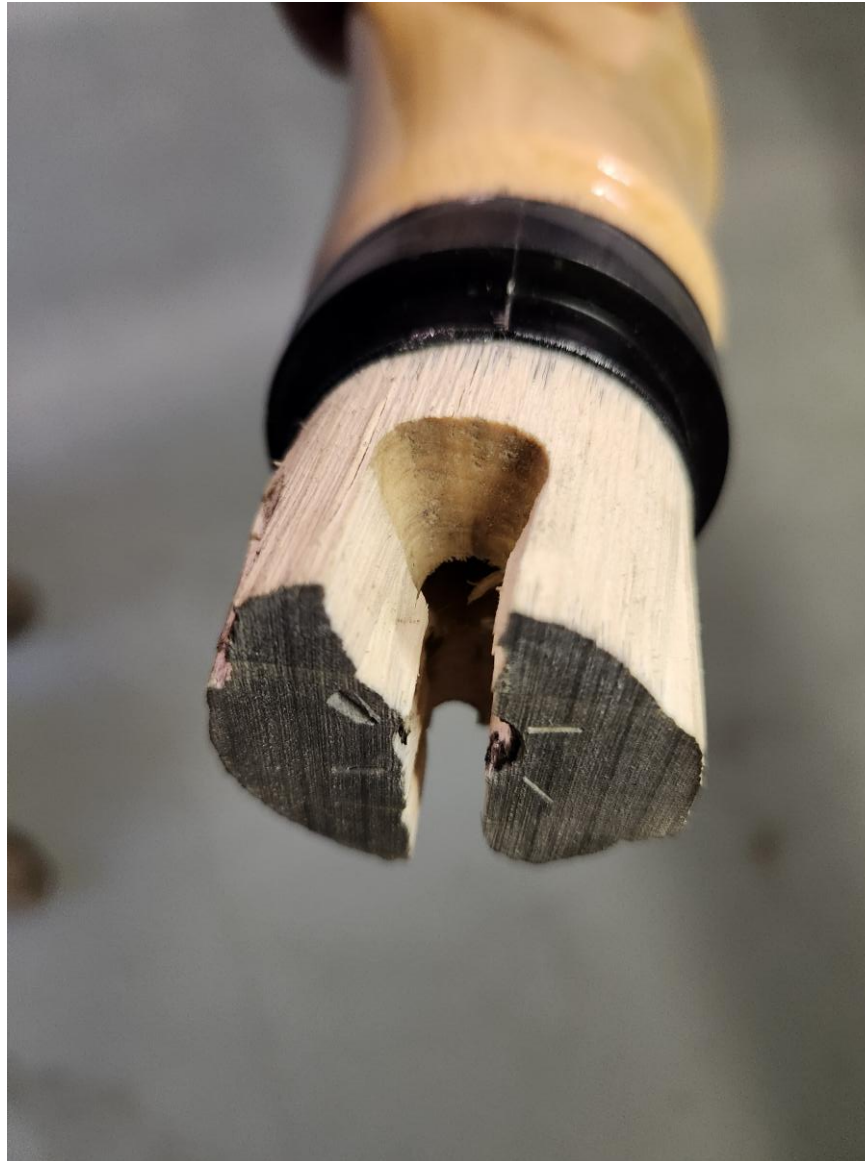
Photograph 3 - Root end of recovered blade. (Courtesy of pilot)
