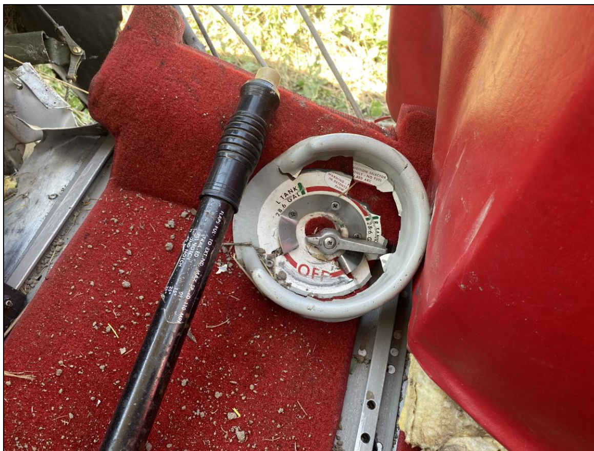
Photograph 4 - Accident site, fuel selector valve. (Courtesy of the FAA)
