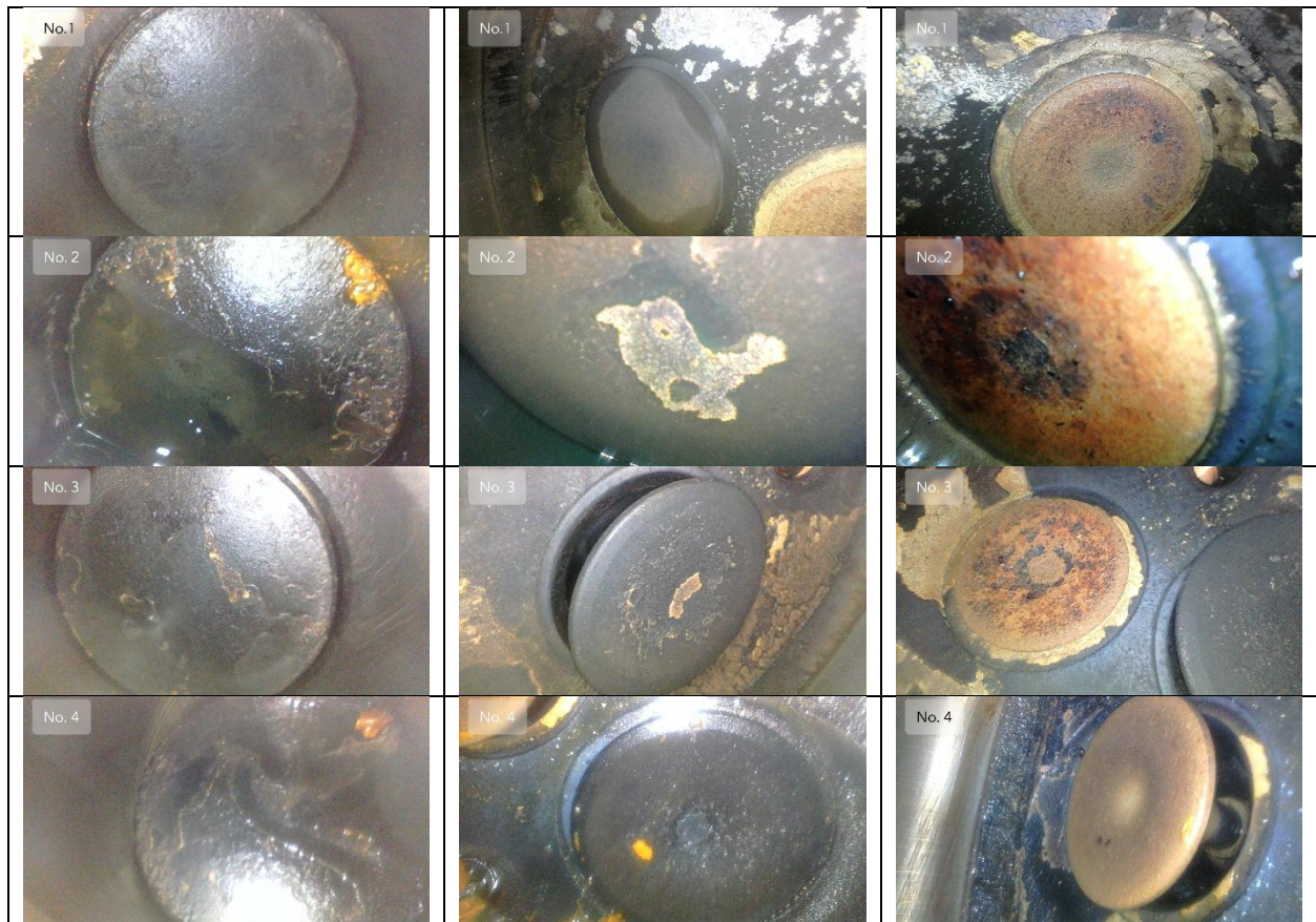
Figure 9-Images of the combustion chambers, piston heads and valves.
