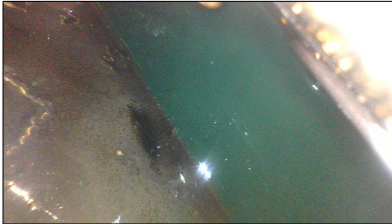
Figure 8-Oil pooled in cylinder No. 2 combustion chamber.
