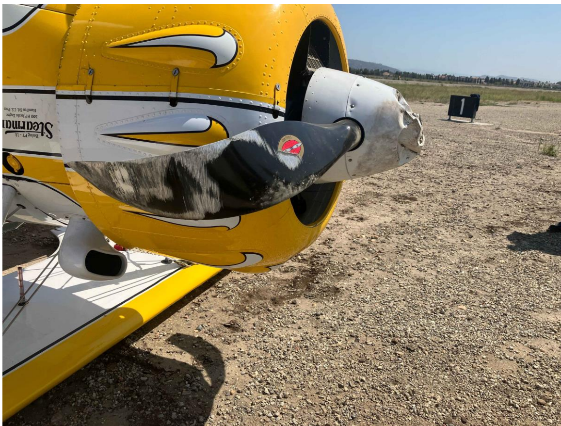
Photograph 4 - Accident site, propeller damage. (Courtesy of CMA Airport Operations)
