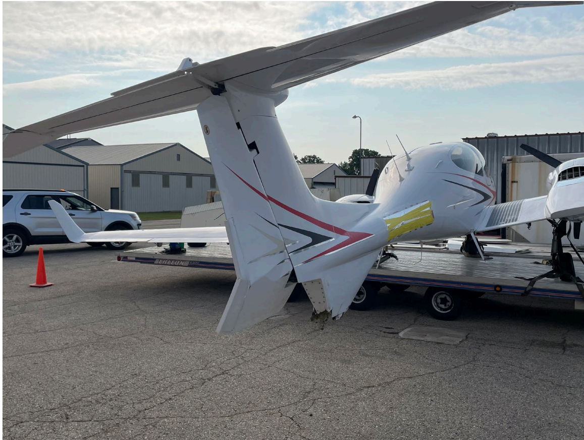
Photograph 2 - View of rudder damage
